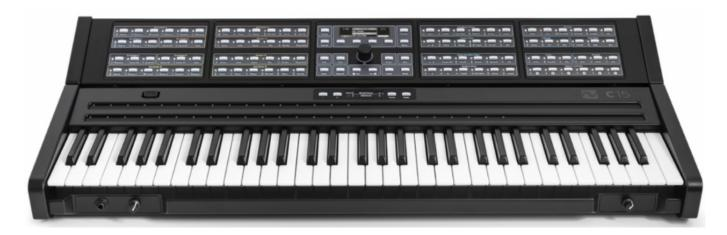
The polyphony of the audio engine has been doubled - from 24 to 48 voices. This gives more resources for layer and unison sounds and strongly reduces the probability of voice stealing. Alternatively, it is possible to run the sound engine with a double sample rate of 96 kHz and a polyphony of 24 voices. This can improve the sound quality and reduce aliasing artefacts.
