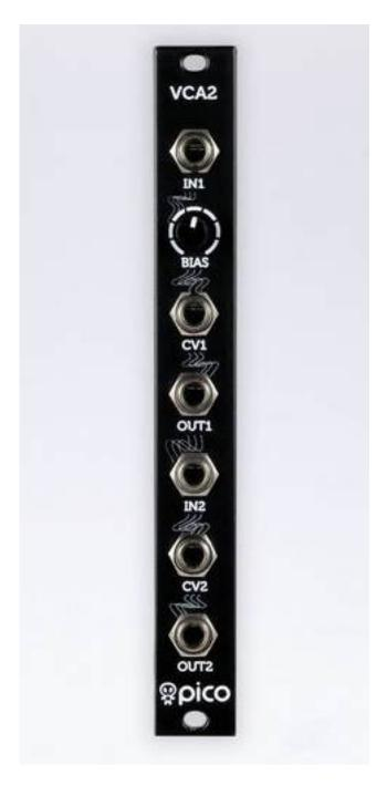
The Erica Synths Pico VCA2 is a compact voltage controlled amplifier module, based on reliable AS3330 chip. It features two independent channels, and the first one comes with the manual offset adjustment, useful for full span vibrato effects. Audio and CV inputs of the first VCA are normalised to the second one, so the module can also be used as a buffered audio splitter. VCAs are DC coupled, and they can be used for controlling amplitude of control voltage signals.
