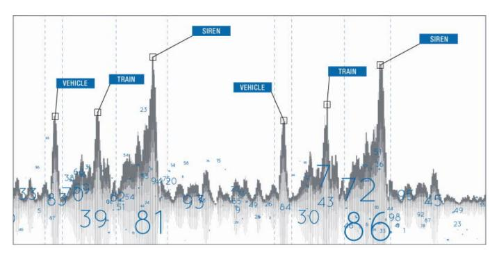
To assist in identifying the cause of a noise level alarm, NoiseScout now provides a text description of the content of the wav files that are recorded during an alarm event. This is achieved using Al analysis and Noise Classification. The text indicates what the possible cause of the alarm could have been, and therefore reduces the necessity to listen to the actual wav file.
