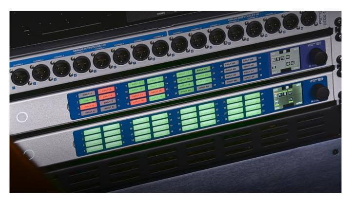
RME announces the M-32 Pro II Series consisting of four new audio networking devices. Each unit consists of a specific combination of MADI, AVB, and Dante and offers either 32 channels of A/D or D/A conversion.
