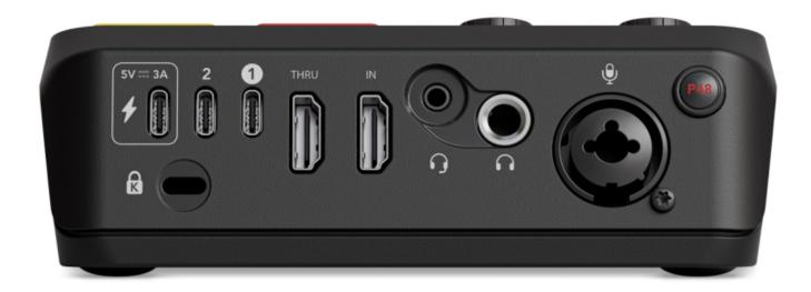
The Streamer X is a revolutionary new product that combines a professional audio interface and video capture card in a compact, easy-to-use console.
