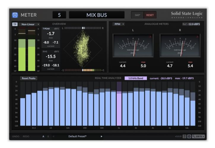
Beyond its comprehensive DAW control, every UF1 purchase includes a perpetual license for the SSL Meter plug-in (worth \$99.99 / £89.99 / €99.99) which is visualised on the large 4.3" IPS display and can be controlled directly from the UF1 surface or the SSL 360° Plug-in Mixer. The SSL Meter Plug-in offers essential metering tools including Peak & RMS levels, K-System, stereo balance, phase corelation bar, Lissajous phase scope, 31-band RTA, VU and PPM metering.
