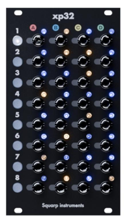
Squarp Instruments introduces the xp32, the ultimate output expander designed to amplify the creative power of the Hermod+ sequencer. With 32 additional assignable CV or Gate outputs, the xp32 transforms Hermod+ into a 16-track CV/Gate powerhouse, an expansive MIDI/USB-to-CV interface, and a versatile preset manager.
