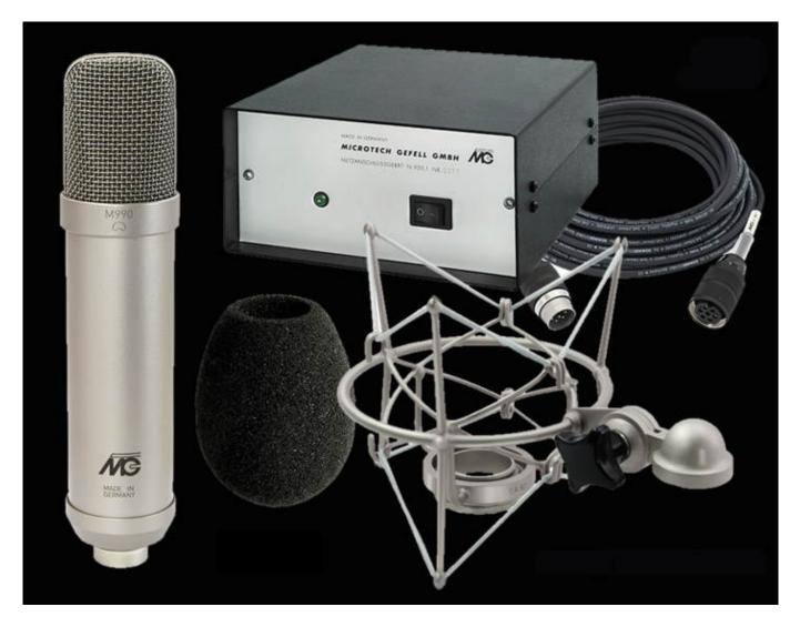
The M 990 is a true, hand crafted microphone that follows Gefell's unique 90-year tradition. This means that everything from hand drilling the back plate, to hand stretching the diaphragm, and individually selecting the capsules and components, to the final assembly and testing is done meticulously, one at a time in both an anechoic chamber and then a live listening test.
