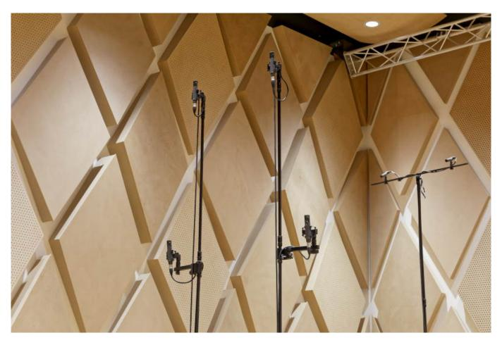
In the TWIN Square array, a runtime-based stereo pair is formed at the front and rear in both the horizontal and the vertical plane. The sound results are impressive and are certainly a match for the cube array concepts that are familiar among sound engineers. However, the square array is much easier to handle and is cheaper to purchase compared to cube arrays with their eight or nine microphones positioned in the form of a cube.
