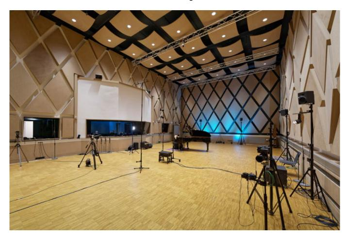
Karl Tessmar is a self-confessed fan of innovative 3D sound worlds, which is why there is nearly always a microphone set-up suitable for three-dimensional recordings installed alongside the conventional microphone arrangement. The microphone array with four Sennheiser MKH 800 TWIN studio condenser microphones goes by the name TWIN Square and was designed and developed by tonmeister Gregor Zielinsky.
