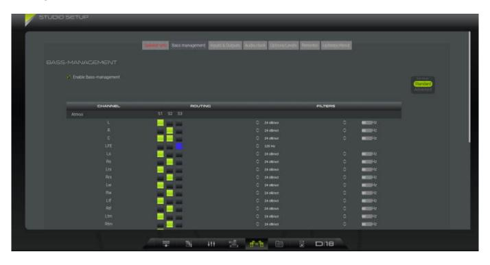
With our Matrix Bass Management, you can bass manage any channel to any combination of subwoofers. The advanced mode allows you to fine tune the crossover filters for each channel.
