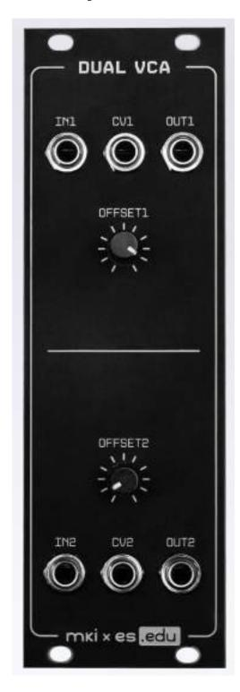
The mki x es. EDU VCA is simple, yet efficient dual VCA for your eurorack system. It has DC coupled inputs, so you can use the VCA both for audio and CV signals. Inputs of the second VCA are normalled to the first one, which allows to split audio signal to both VCA or control both VCAs with a single CV. A 60 page build manual explains electronics behind the module and provides step-by step build instructions.
