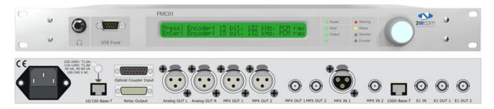
The FMC01 is groundbreaking compact codec for high-quality FM MPX distribution via IP with synchronization in microsecond range and short delay. The device allows 100% loss less audio encoding and decoding of MPX audio bands (mono, stereo). To ensure best signal quality, the codec is equipped with a high-end converter (ADC, DAC) and supports sample rates of 132 -192 kHz with 16, 20 or 24 bits resolution.
