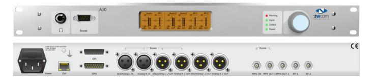
Since launch in 2016, the versatile monitoring receiver is equipped with a wide range of highly user-oriented monitoring functions, which enables operators to monitor single or multiple transmitter frequencies. Right from the beginning, the A30 has offered a number of interfaces including analog or digital audio input, MPX input, two analog or digital audio MPX outputs, GPIs, SNMP and two parallel MP3 streams.
