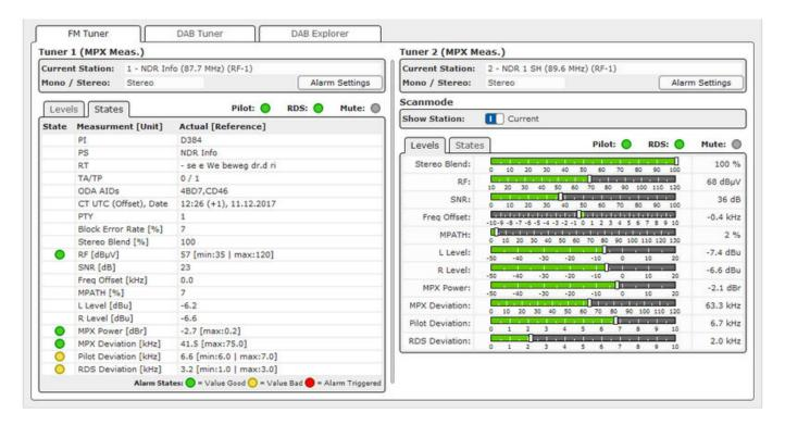
In addition, the second tuner implies the function scan-mode (Round Robin) to monitor up to 30 frequencies. The configuration of all FM/RDS parameters and the sequences of the monitored stations can be handled individually via web interface. In case a value does not comply with the pre-settings, an alarm is forwarded via SNMP, Email or relay. All alarm activities are stored in a separate archive with time stamp, type of alert and the equivalent frequency.
