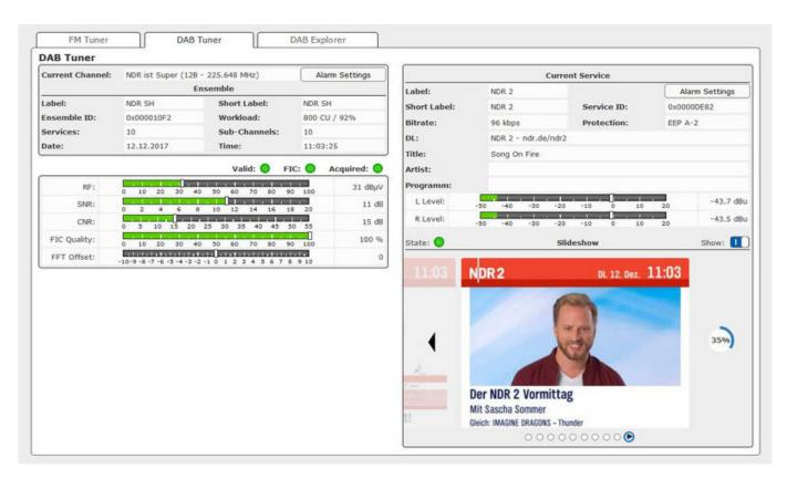
This new feature enables operators to monitor DAB+ signal parameters such as RF level, FIC quality, audio level and the slightshow (SLS – displaying all included categories). The integrated band scan simplifies the setup for DAB+ monitoring by automatically detecting for which frequencies a MUX signal is available.
