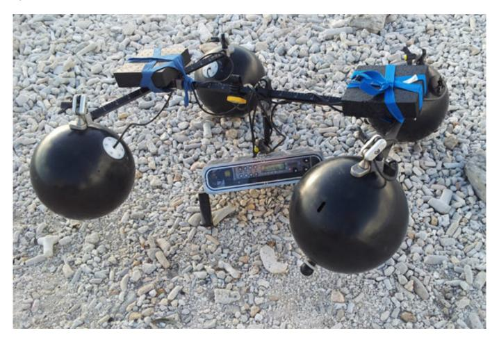
Five TC4042 hydrophones (the DS spheres) have been used, three TC4013S with the camera housings and one TC4032 to record distant signals. Recordings were made with a Sound Device 788T in 24-bit 48kHz
