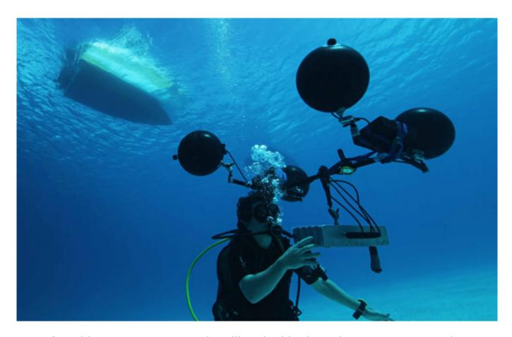
One of our biggest concerns was handling the big rig underwater. However, it turned out that the calculations were correct and the 25-pound rig with two buoyancy devices was tared perfectly neutral. Thus even a relatively inexperienced diver was able to handle this colossus without problems.
