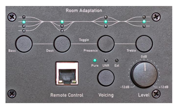
In this context, the "Pure" setting stands for the basic sound tuning of the current A-Series, while "UNR" activates a legacy mode with the classic playback curve of the superseded X-Series, so to speak. The Ext(ern) setting can be used to load a profile created using the SoundID Reference room correction software from Sonarworks. In addition to the obligatory gain control (-12dB to +12dB) and balanced (XLR) and unbalanced input (RCA), the A-Series also has an RJ45 network socket.
