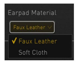
We had already mentioned that an optional textile headphone cushion set is available in addition to the standard leather set. The different materials of the ear pad also have an acoustic influence, so you can specify the type of pad used in the plug-in to compensate for this influence using an appropriate equalization curve (see figure above).
