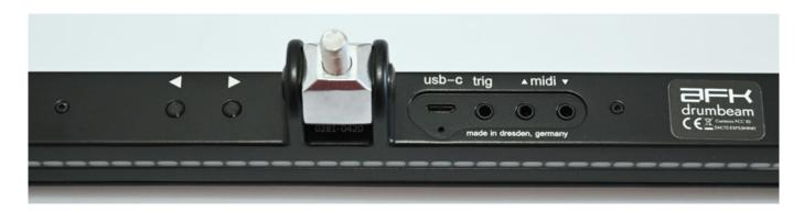
Now let's move on to the connections. At the bottom is a USB-C port for a power supply (at least 0.4 amps) and for future firmware updates. The 3.5mm trigger jack can be used to connect an external piezo sensor, which can be used to trigger a kick drum via a foot pedal. This input is optimized for Roland KT models. There is also a MIDI input and output in the form of 3.5mm TRS jacks with A-type format assignment. Two buttons allow you to select eight presets from the current preset bank.
