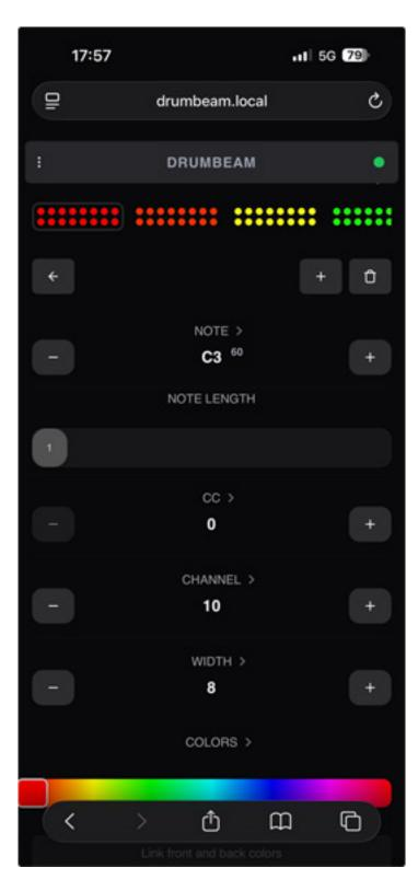
On the preset's start page, the user can select or trigger one of the segments and then change the settings for that segment, such as MIDI CC value, note, note length and channel, segment width, LED colors, velocity range and curve, and CC range and curve. Incidentally, the last screenshot was taken on an iPhone running iOS 26.
