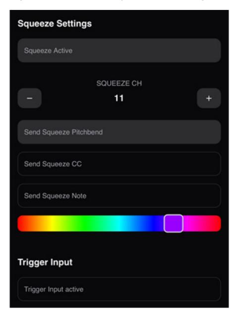
Particularly noteworthy is the optional "Squeeze" function, which allows Drumbeam to be controlled by hand. This also allows CC data or pitch bend data to be sent. When this function is activated, the area changes color when you place your finger on it. The color of the LEDs can also be set separately for this case.
