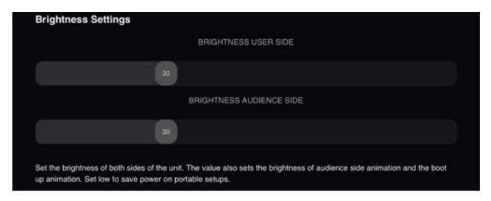
The brightness of the LEDs on the front and back can even be adjusted separately
