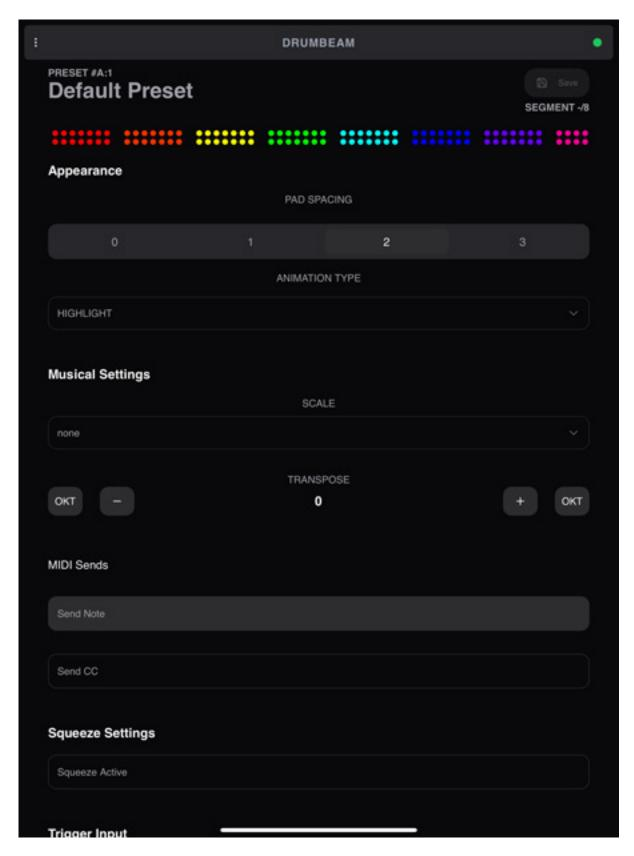
After connecting to the Wi-Fi, you will be taken to a page with global settings (see image above). Here you can set, for example, whether MIDI notes or CC should be transmitted. You can also set how the LEDs work. The default LED mode is that the
