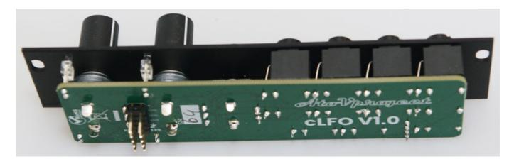
The operating current of the 6-HP wide module is relatively low at 49mA peak (+12V) or 57mA peak (-12V). The front panel is made of aluminium. The module is available with either a black or silver front panel.
