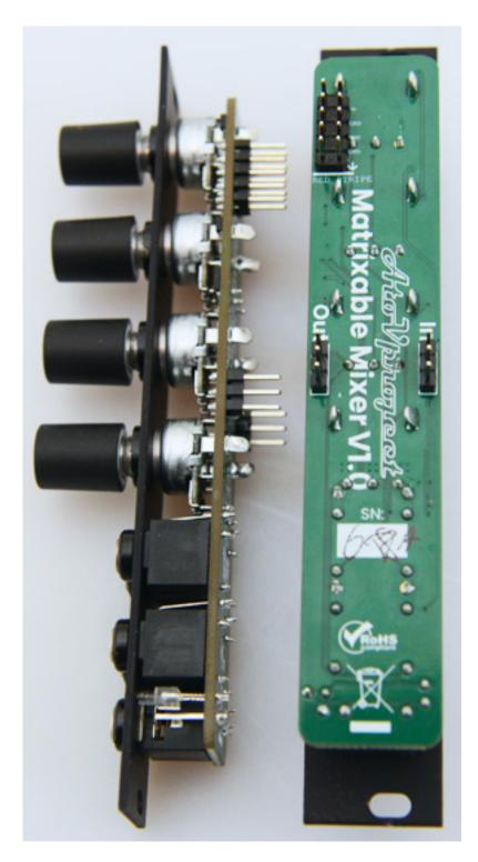
However, several mixers can also be cascaded. Cascading is realised via a three-wire cable. For this purpose, the modules each have an In- and Out- terminal strip (see illustration above) on the rear of the circuit board. Two connection cables for module connection are provided with the Duo. For cascading, the Out port of the first mixer must be connected to the In port of the second mixer. The operating current is 10mA (+12V) or 8mA peak (-12V) per module.
