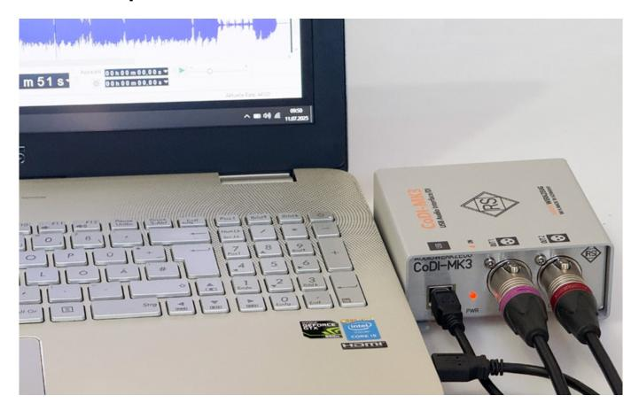
There were no problems when connecting to computers. The connection was always established immediately under various operating systems. Of course, we also tested the sound with various materials and under realistic conditions with a headphone amplifier and long cables. We can attest to the converter's high linearity and, above all, its excellent reproduction of transients.
