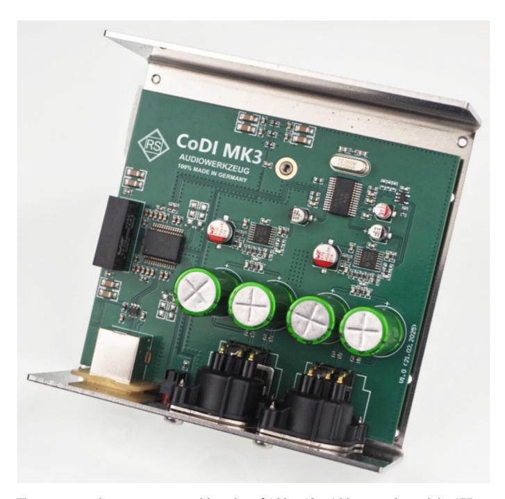
The converter is very compact with a size of  $100 \times 42 \times 100$ mm and a weight 475 grams. It is powered via the USB interface. A red LED serves as an operating indicator. No drivers need to be installed, as the device operates in Class Compliant Mode. It can be used on computers running Windows XP (i.e., not only 64-bit but also 32-bit operating systems), Mac OS 10.4, and Linux from Kernel 2.6. The CoDIMK3 needs only 76mA with a load of 600 ohms at the outputs.
