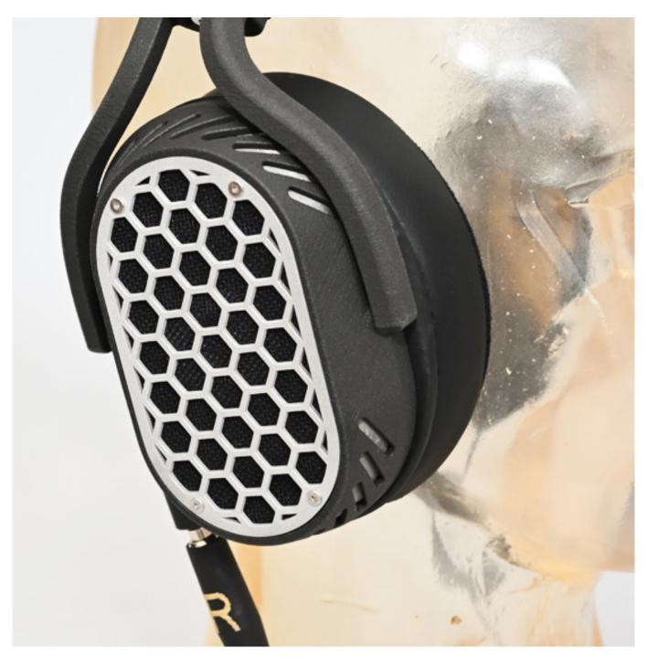
A 50 mm dynamic driver with a relatively low nominal impedance of 20 ohms (@ 1kHz) is used. The manufacturer specifies a frequency range of 10Hz to 20kHz. A passive electrical filter is used in the headphones to adjust the bass and treble. Headphones are usually tuned purely acoustically. The rear of the ear cups is acoustically very open (see image above).
