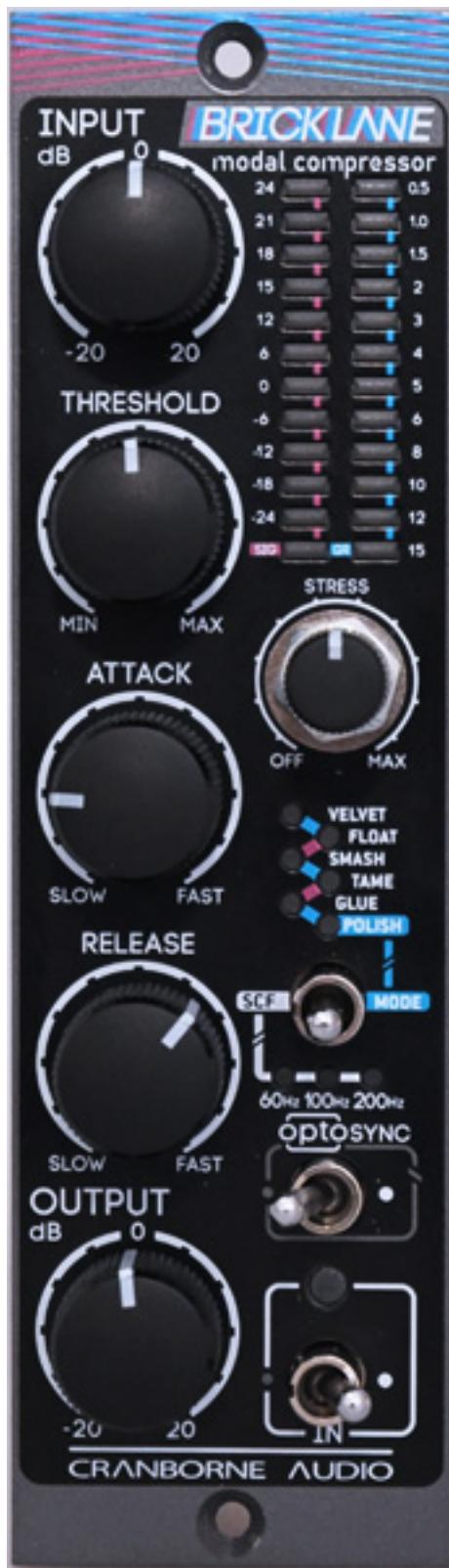
At first glance, the controls of the Brick Lane 500 look very familiar. On the left are the knobs for input, threshold, attack, release, and output. The labels and scales are well chosen. A toggle switch at the bottom right activates the compressor, while another activates the (opto) sync.
