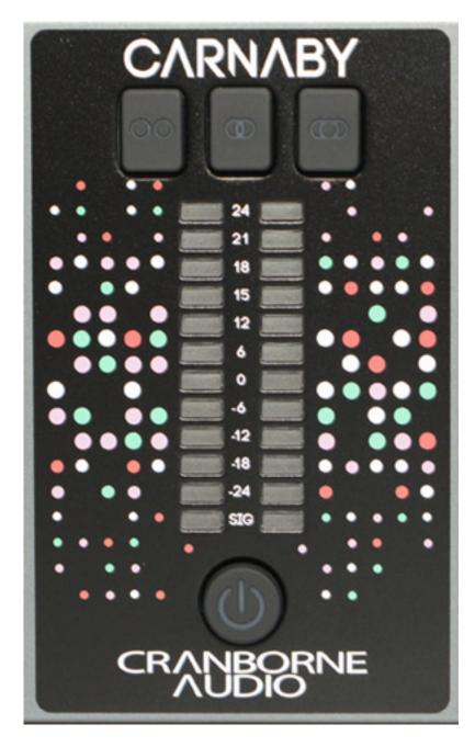
The features are complemented by a large LED display with a peak hold function and an on/off button. The mains switch on the back can therefore remain on.
