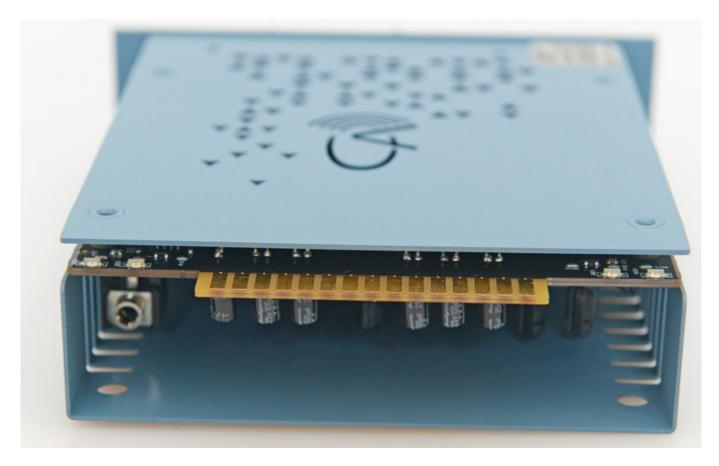
The cover of the Legacy Edition can be removed by loosening four screws – and reassembled with a little fiddling. Overall, the construction makes a solid impression, and the controls are exemplary but very densely packed. Inside the unit, there is a DIP switch strip that can be used to set some "utility" settings, including how the LEDs and bypass switch work.
