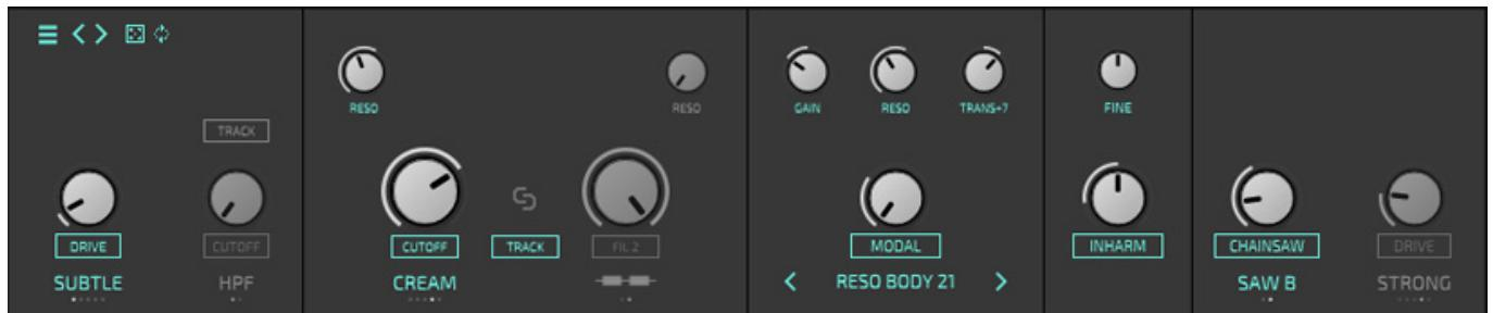
The third section provides access to the downstream filters, a high-pass/notch filter, and two low-pass filters that can be connected in parallel or in series.
