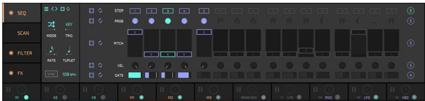
The step sequencer, with its operating modes Forward, Backward, Ping Pong, and Random, offers step-by-step adjustment of probability, pitch, velocity, and gate length. Each step can be activated or deactivated individually, and the loop length can be changed individually for each parameter.
