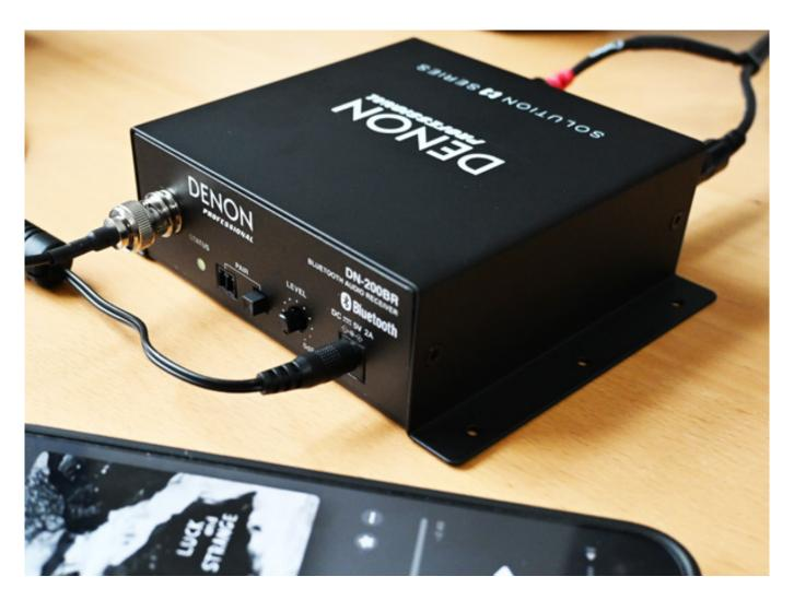
After connecting the device for the first time, the LED flashes and the device waits for a Bluetooth connection. We used an iPhone 15 Pro Max with iOS 18.2, selected the DN-200BR in the Bluetooth dialog, and the connection was established immediately.
