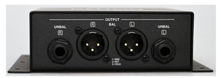
The output level is -2dBu for the unbalanced output and +4dBu for the balanced output. According to the manufacturer, the signal-to-noise ratio is >75dB, and the transmission range is 20 Hz to 20kHz. The THD is specified as > 0.01%.
