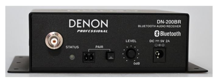
The power connector, BNC antenna connection, and a pairing button are located on the front panel. Interestingly, there is also a socket for the pairing button so that an external switch can be used. The audio output level can still be adjusted using the LEVEL control. A status LED indicates whether the device is switched on (flashing) and whether a Bluetooth connection has been established (steady light).
