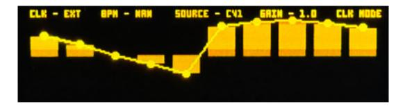
The clock modulation menu is also interesting. Here, you can set a clock source (internal/external), the speed in BPM of the internal clock, the modulation input source (CV1 or all), and a degree of modulation. With an incoming or internal clock pulse, the input value is stored as a sample & hold and assigned to the current filter. With each clock pulse, the corresponding filter number will increase.
