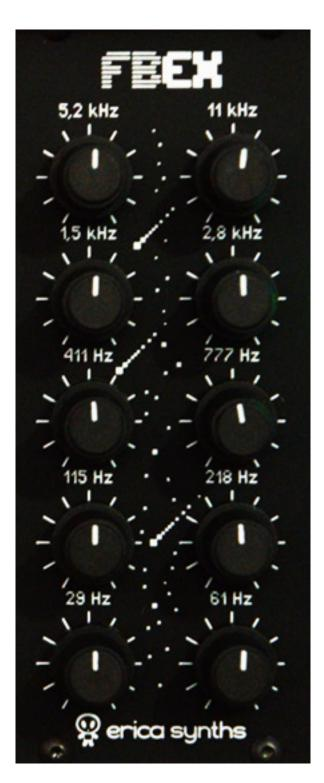
The expander is self-explanatory. The target frequencies of the bands are displayed above the controllers. The ten potentiometers are used to set the gains of the ten bands. As mentioned earlier, there are two operating modes: Offset, where the values are added to those of the filter module, or Attenuate, where the expander settings act as attenuators.
