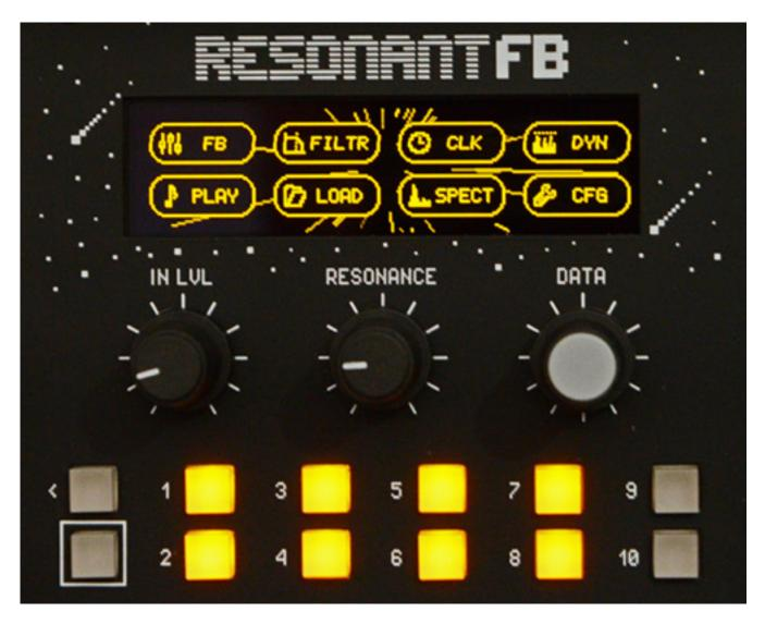
This module is operated via twelve buttons with LED indicators, a controller for adjusting the input level and filter resonance of all bands, as well as a push/turn control for menu selection and parameter entry. A monochrome OLED display measuring  $70 \times 18 \text{mm}$  is included.
