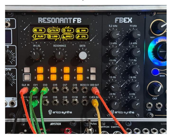
We had a module with firmware 1.2 that we updated to the firmware version 1.3. The update is done by an audio file that is provided on the Erica Synths website. This works best if you play the audio file on a laptop or PC and connect the audio output of the PC directly to the IN socket of the filter module because if you route
