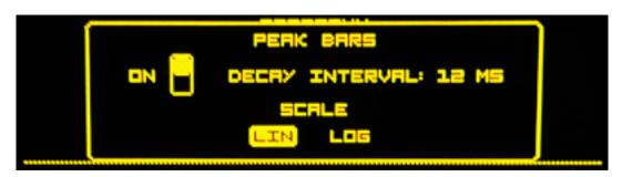
By default, however, it is set to LIN, which means linear; therefore, the display only takes place in a small area on the left. Thus, it is advisable to switch to logarithmic (LOG) if necessary.
