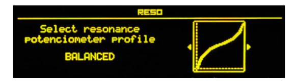
RESQ allows you to adjust the resonance control curve. In addition to the standard BALANCED setting (see figure above), you can select various linear (linear only upper, only lower or complete control range) and logarithmic curves (normal and inverted).
