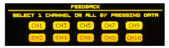
It is interesting to note that you can determine which filters are used for resonance feedback. This can be set globally via the feedback submenu, either all, none or one of the ten filter bands.
