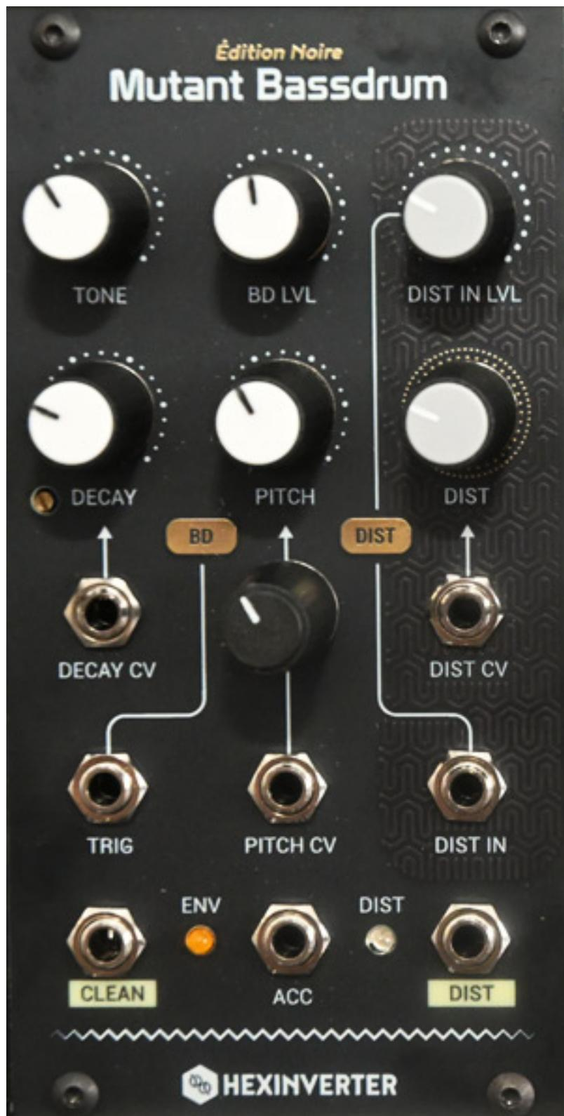
The “Mutant Bass Drum” is based on the circuit design of the TR-808. A pulse with a length of one millisecond is sent to a T-network consisting of resistors and a capacitor, generating a sine wave with decreasing amplitude. A notable feature of the original circuit is that when a trigger with accent is used, not only is the volume
