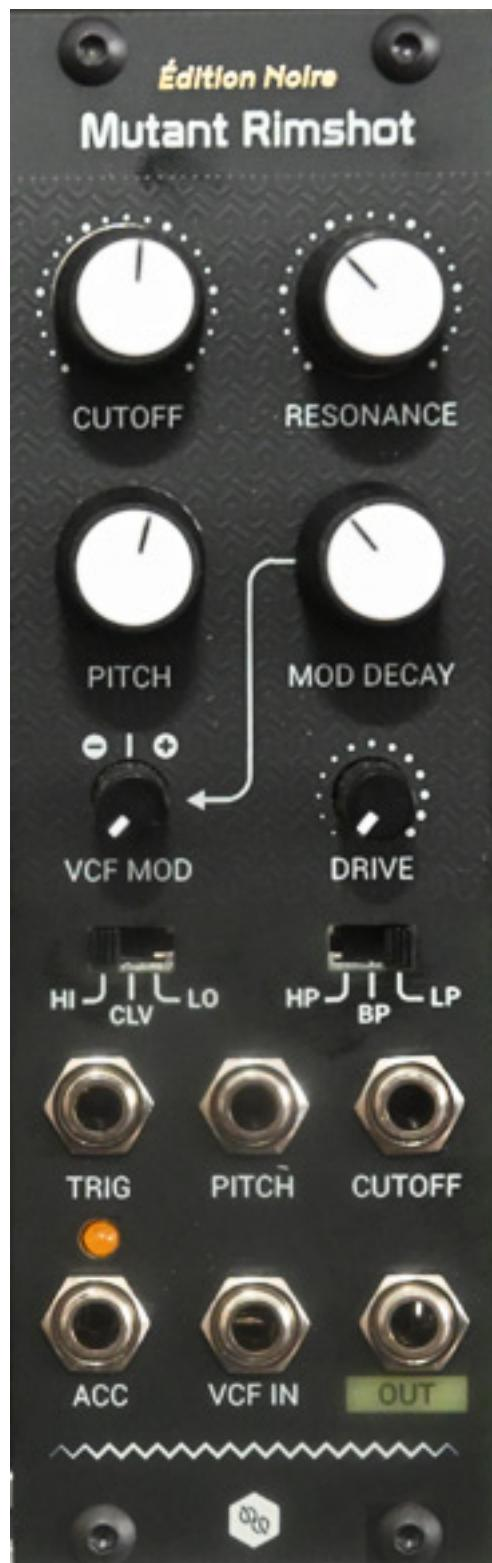
With the exception of the narrower 8 HP wide "Mutant Rimshot" module, all modules are 13 HP wide. The concept of the "Mutant Rimshot" module is again inspired by the TR-909 and is based on three oscillators formed by a pulse and an excited bridged T-network, as well as a downstream state-variable filter (switchable low-pass, band-pass, and high-pass) for sound shaping. The VCF IN jack allows an
