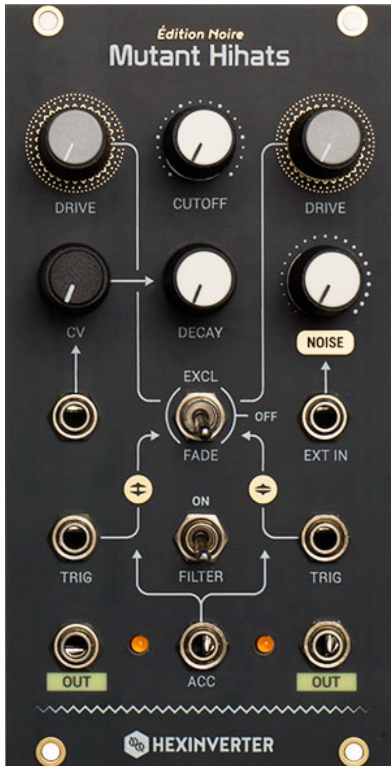
The Mutant Hi-Hats module was again inspired by the TR-808 in some respects. However, instead of the transistor-based circuitry of the TR-808, more modern low-noise op-amps or OTAs are used here. We tested the version from Hexinverter and not from Erica Synths, as we already had the module available. There are no differences in sound whatsoever. The module offers a trigger input for both the
