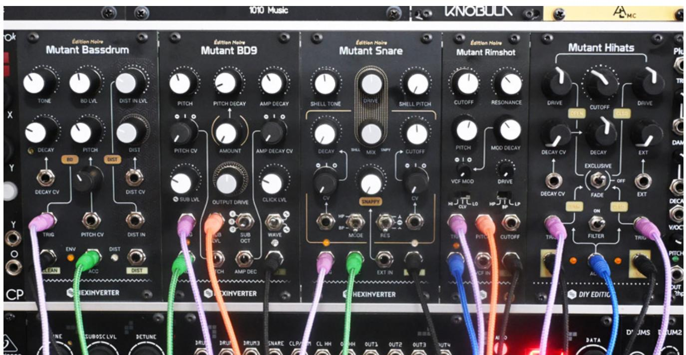
The modules' operating current is very low. We measured the highest current on the Mutant Snare at 67mA (+12V) and 62mA (-12V). On the Mutant Bassdrum, it was only 20mA (+12V) and 17mA (-12V).
