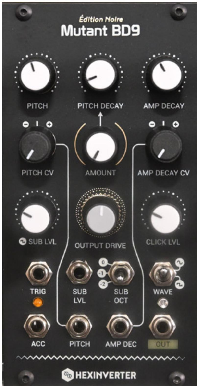
The "Mutant BD9" bass drum is an alternative to the previously presented "Mutant Bassdrum." It is based on the bass drum of the TR-909 with its typical sine waveform, but it can also be switched to a square waveform as the signal source using the WAVE switch. The pitch can be adjusted in the range from 30 to 240Hz. Unlike the Mutant Bass Drum, the pitch can be modulated using a separate
