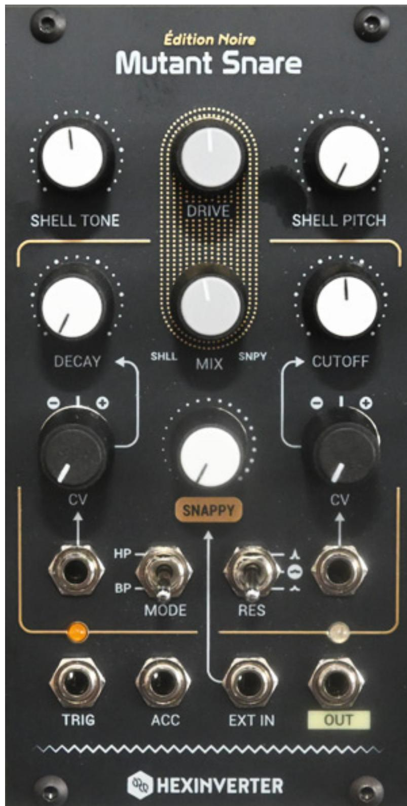
The “Mutant Snare” is again conceptually based on the TR-808. The snare sound is generated by two sine oscillators (shell component), one of which can be detuned, and a noise generator (snappy component). Instead of the internal noise generator, an external noise signal can also be fed in (EXT IN). The level of the external or
