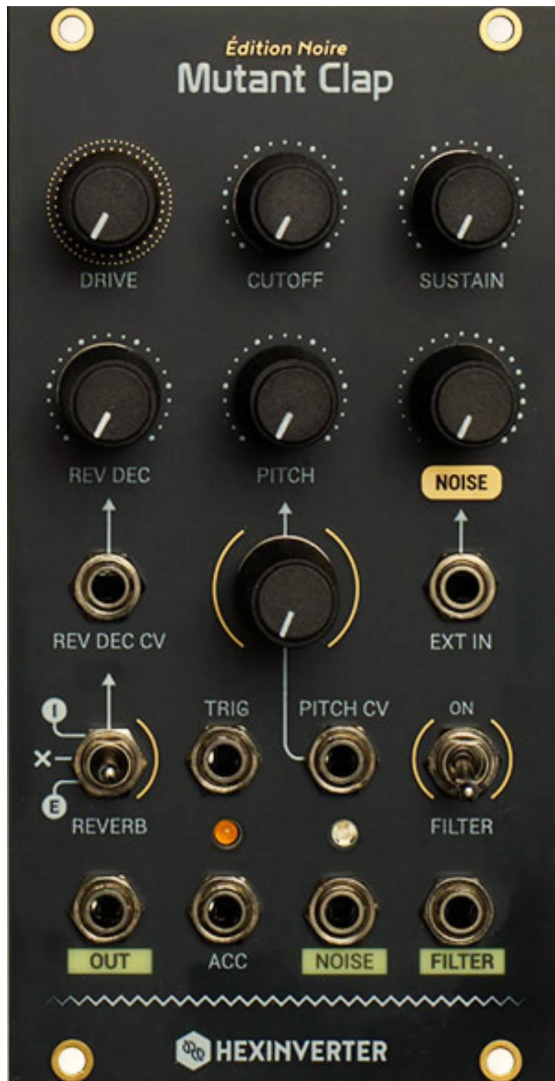
We did not have the "Mutant Claps" module available for testing, but we would still like to briefly mention it. Mutant Claps is inspired by the TR-909. The pitch can be adjusted via PITCH, the filter frequency of the bandpass via CUTOFF, the decay time via SUSTAIN, and the level and distortion via DRIVE. In addition to trigger and accent input and audio output OUT, the pitch can also be modulated via the PITCH
