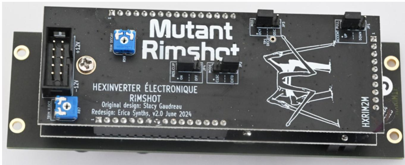
On the rear panel of the Mutant Rimshot module, there are four jumpers that allow the user to perform various preconfigurations. More on this later.
