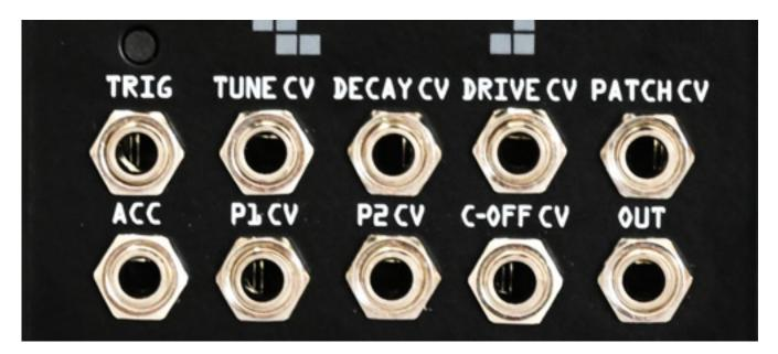
Now let's take a look at the ten inputs and outputs. In addition to the monophonic audio output, there is a trigger and an accent input for emphasis (plus 2dB). Above the trigger input, there is also a small button for manual triggering. Furthermore, all six adjustable parameters can be modified using control voltages.
