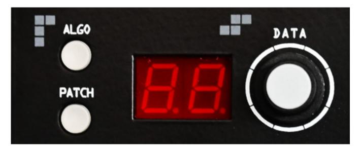
When an algorithm is displayed, you can switch between "Mono" and "Poly" play modes by pressing the rotary encoder. In Mono mode, a new trigger starts a new voice, and the previous one stops. In Poly mode, the triggered voice continues to be played, and the new voice starts. Up to four voices can sound simultaneously in Poly
