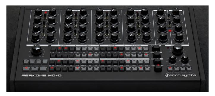
Let's take a closer look at the user interface of the Perkons HD-01. The pattern sequencer is located at the bottom, with four voices and a master section at the top.
