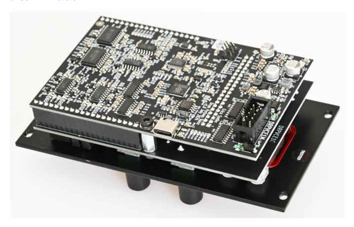
The power consumption is approximately 55mA with a +12 volt power supply and approximately 3mA with -12 volts. On the rear panel, next to the power connector for the module, there is a USB-C socket for connecting to a computer to update the module's firmware. The audio output level is 10 volts peak/peak, and the CV input voltage range is -5 to +5 volts.
