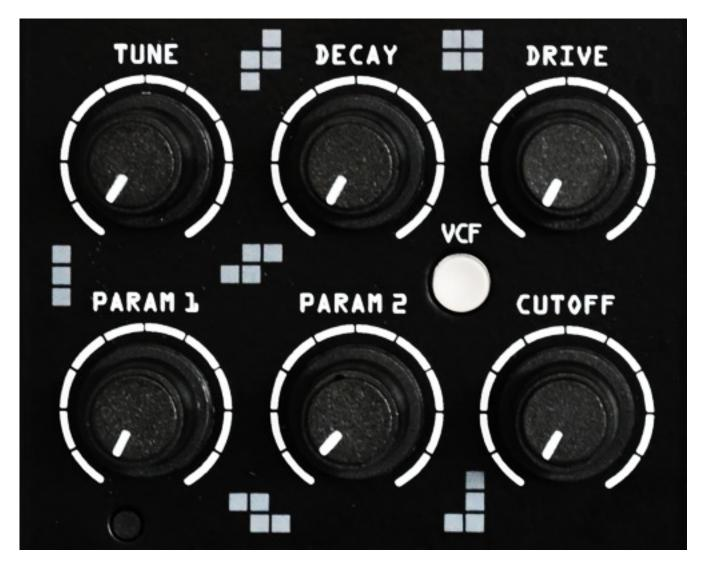
Below are six knobs for pitch, decay time, level or drive, filter frequency, and two parameters that change depending on the selected algorithm. For algorithms A1 to A3, for example, these are the size of the pitch envelope or the degree of modulation. In the first version of the manual, the description of parameters 1 and 2 for algorithm A appears to be reversed.
