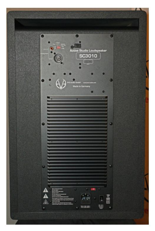
The two analog inputs have an impedance of 10 kiloohms. Either an RCA (unbalanced) or a 3-pin XLR socket (electronically balanced) is available as an input. The maximum input level can be switched between +7 and +22 dBu, which corresponds to the usual nominal levels of -10 dBV or +4 dBu with corresponding headroom.
