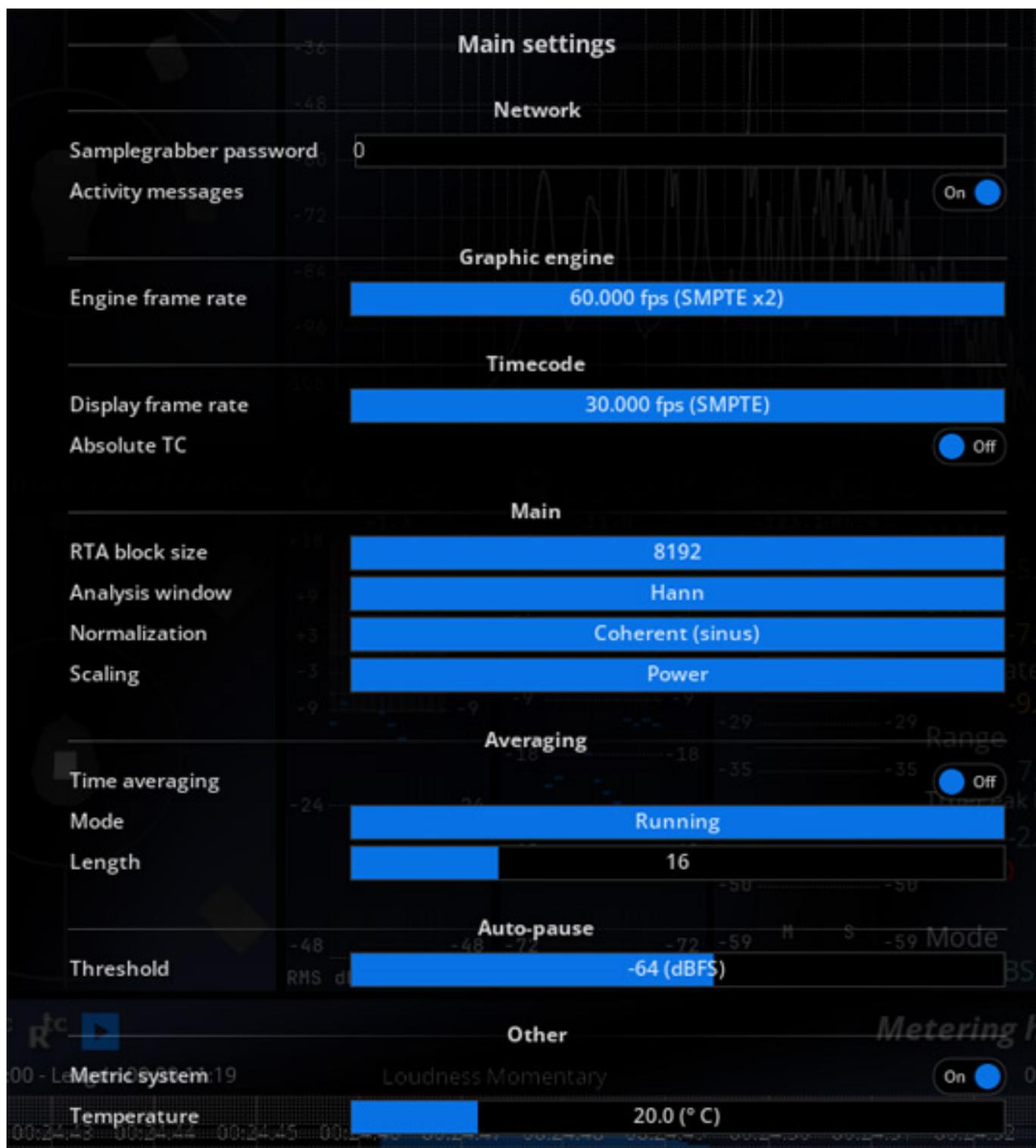
In the main settings (accessible via the gear symbol), display frame rates and basic analysis parameters can be adjusted.
