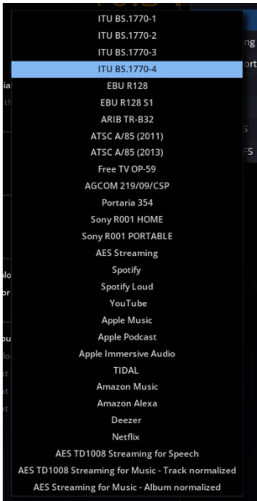
A whole range of different measurement methods is available for loudness measurements (see figure above). Dolby Atmos is not included in the selection. This is because loudness measurement is realized through a downmix, and it is best to use the Dolby Atmos renderer for the loudness Dolby Atmos value.
