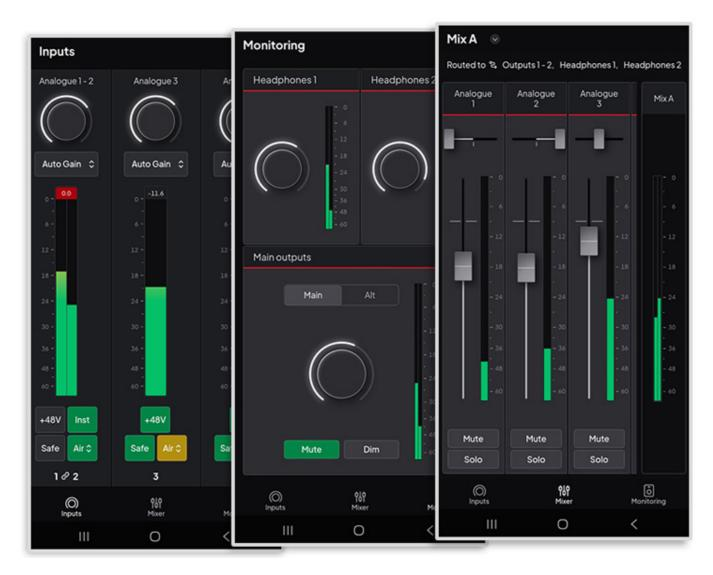
Remote control of parameters using the app proved to be very practical. After downloading it from the App Store, the connection via a QR code was quick and smooth. Channel inputs and outputs, as well as levels for headphones and monitor output, can be controlled.
