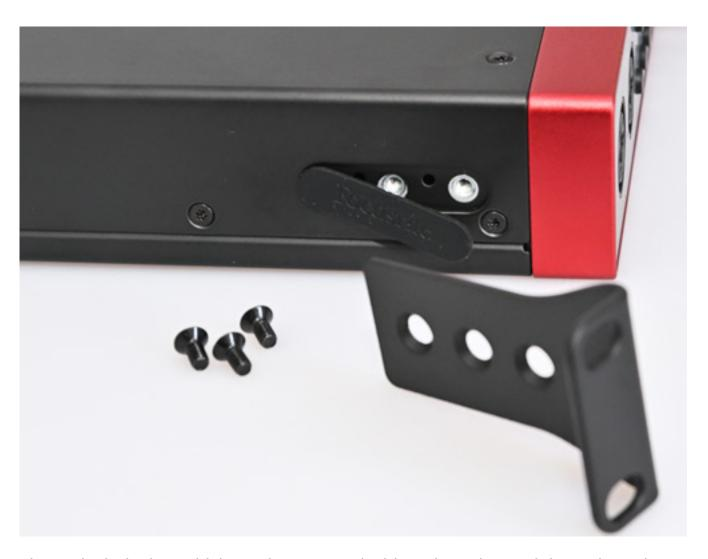
The 19-inch device, which can be mounted with rack angles, weighs 3.3kg. It has a height of 1U and a depth of 260mm. The threads for attaching the metal angles are hidden behind a rubberized cover for desktop use.
