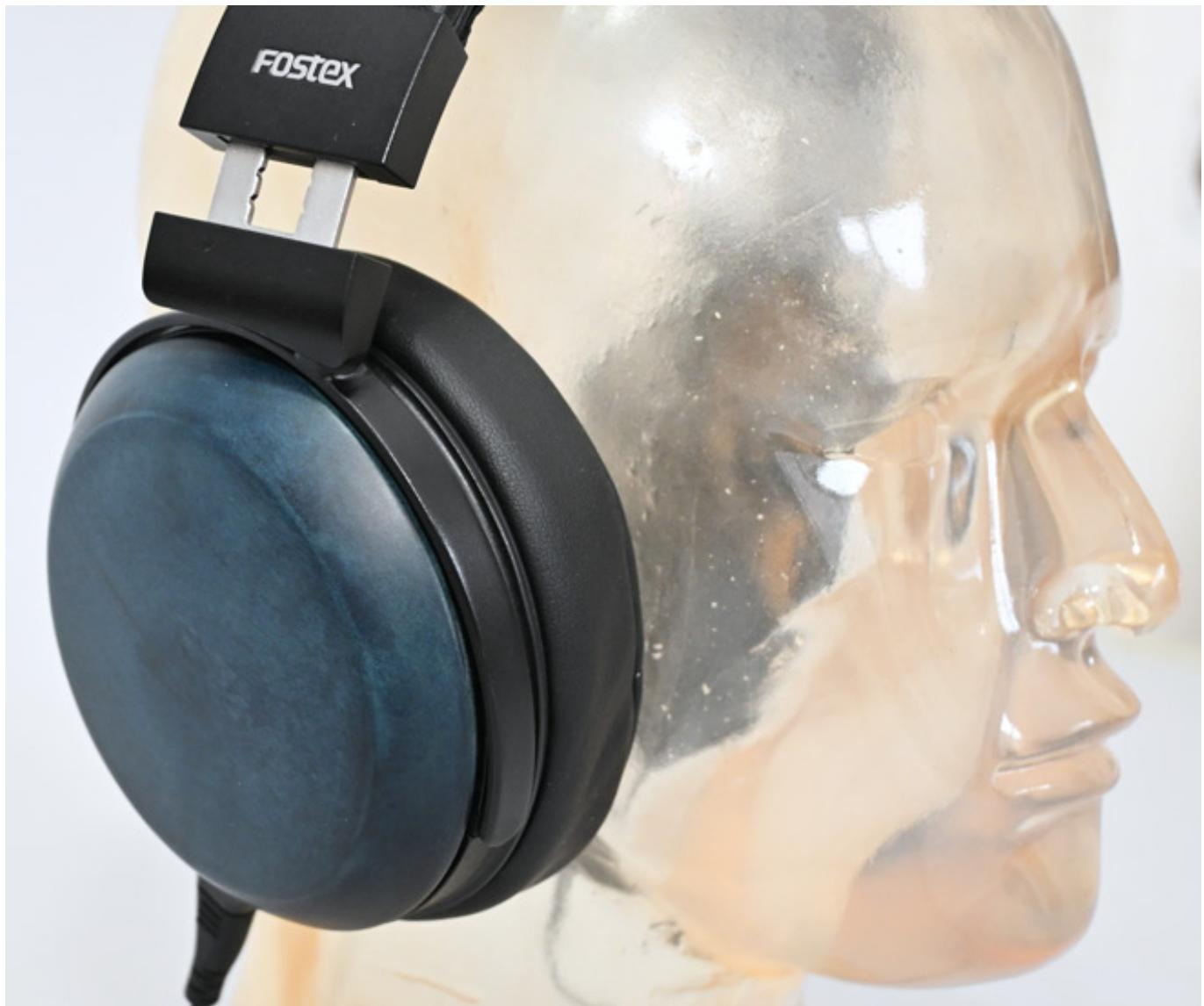
Now a few words about the magnetostatic drivers. Unlike a dynamic driver, the coil does not move in a permanent magnet to drive the diaphragm; instead, the coil is located on the diaphragm itself. This design results in significantly less mass that needs to be moved, allowing the diaphragm to follow the electrical input signal with greater precision. Consequently, there is less overshoot or overswing due to inertia, leading to greater linearity.
