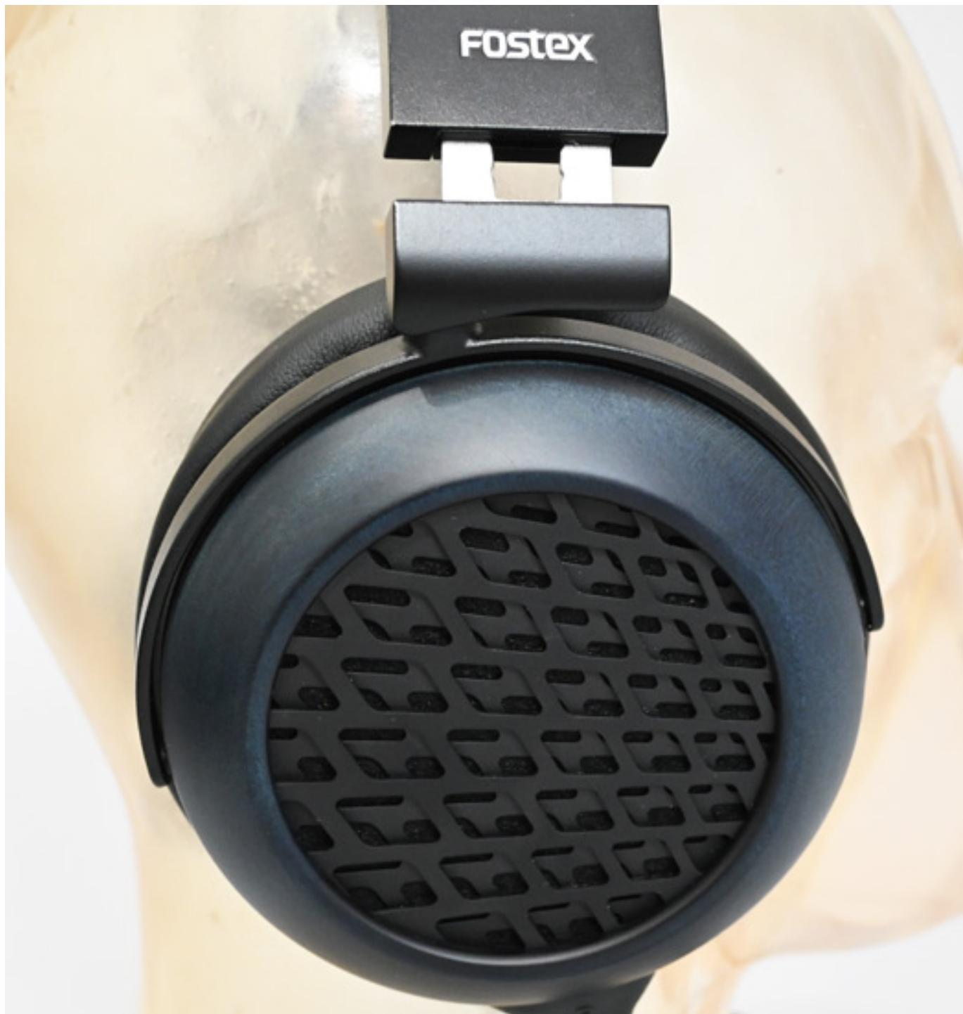
Let's start with the technical data. Both headphones feature the same driver. The impedance of the headphones is 32 ohms, which is very low, as is the case with many modern headphones. The maximum input power is specified as 3 watts. Fostex specifies a frequency range of 10Hz to 40kHz. The sensitivity of the open TH1100RP (see figure above) is 96dB/mW and that of the closed TH1000RP (see figure below) is 100dB/mW.
