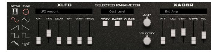
An extended LFO (XLFO) is offered here, and it offers many optional possibilities, such as a delay during use, various waveforms, sample & hold function, phase adjustment, etc. There is also an extended ADSR envelope generator with settings
