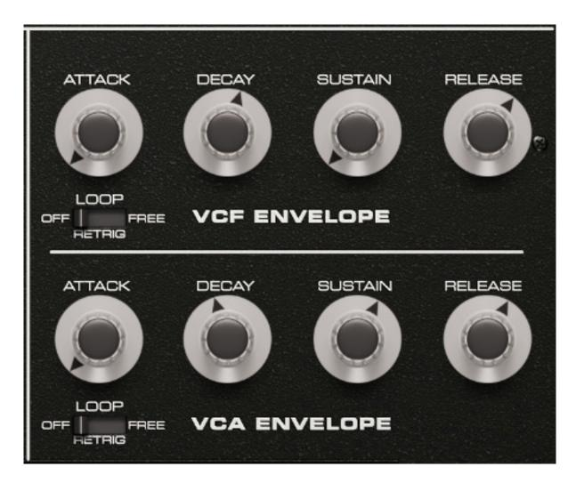
The two envelope generators can also be operated in loop mode, with and without retrigger when a button is pressed.
