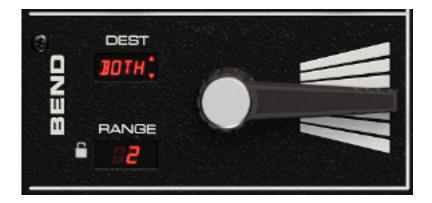
The virtualised wheel is also modelled on the original, and it offers several operating modes, and its modulation range can be limited on the virtual instrument.
