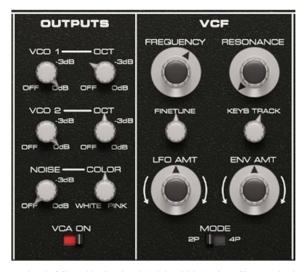
A mixer is followed in the signal path in which a sub-oscillator and coloured noise can be added in addition to the oscillators. The filter is another striking feature of the OB-1 in terms of sound, with fine-tuning control in addition to the main frequency control. The original OB-1a does not have this control. As with the original, the low-pass filter can be switched to two-pole (12 dB/oct.) or four-pole low-pass (24 dB/oct.).
