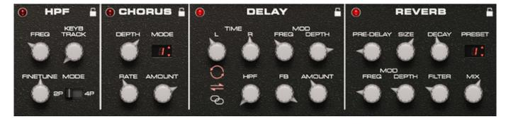
On the right-hand side, the extended display offers four effects: a high-pass filter with keyboard tracking and 2/4 pole switching, a chorus, a delay with modulation
