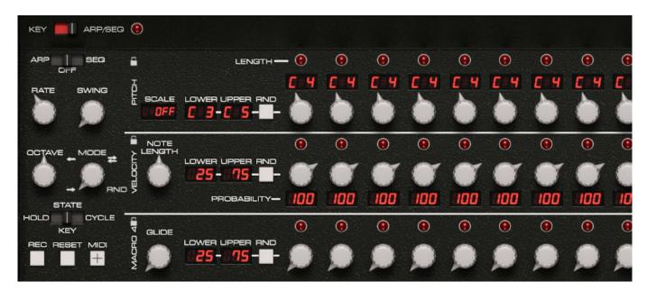
The GForce OB-1 also has an integrated arpeggiator and step sequencer (maximum 16 steps). If the STATE parameter is set to CYCLE, the sequencer is synchronised with the DAW tempo. In addition to pitch, the velocity can be set for each step, and the value of MACRO 4 can also be influenced for each step in a third row. The note length and glide value can also be set globally for the entire sequence.
