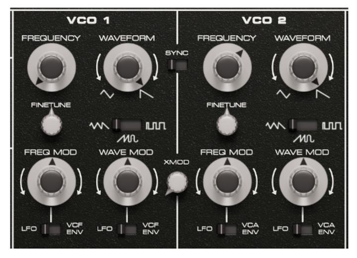
LFOs or envelope generators can be connected to the frequency and waveform. A hard sync function is possible between oscillators 1 and 2. There is also a cross-modulation, which - also in contrast to the original - cannot only be switched, but also be continuously adjusted.
