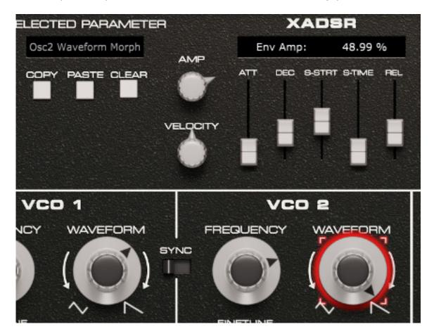
Switching the XLFO/XADSR to a parameter is very simple. The control is selected with the mouse, and the parameter name then appears in the SELECTED PARAMETER output field, and then you only have to make the corresponding settings. The modulation index can be set for the XLFO using the AMT fader and for the XADSR using the ATT fader. The modulation index is then symbolised by a red ring that varies in its intensity. This is also visible when you exit the extended display mode.
