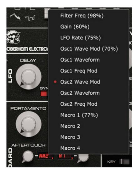
After Touch and Keyboard Velocity can be routed individually to various parameters, including one of the four macros.
