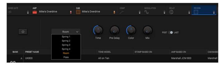
Effects, amps, and cabs can be selected and set in the header area, as with the TONEX software (see figure above). As soon as you change a parameter, this change is also made in the connected pedal - and changes made to the pedal are also synchronized in the software in the opposite direction.
