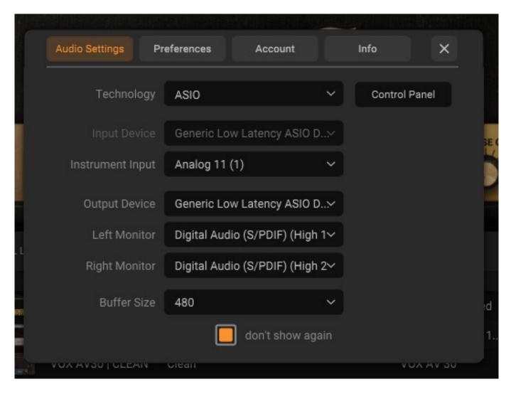
With the stand-alone software, the audio interface and outputs can also be specified. ASIO drivers can also be used here (see figure above).
