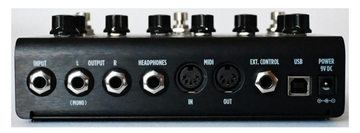
Not only does the internal processing work with 24 bits at a sample rate of 192 kHz, but also the A/D and D/A converters. The TONEX pedal offers a mono input and a stereo output, all equipped with a 6.3mm jack plug, as well as a MIDI interface with input and output, an external controller connection (expression pedal or foot switch), and a USB connection for optional connection to a computer for use by an editor or for firmware updates.
