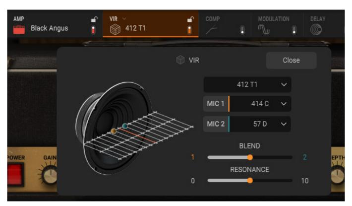
The cabinet can be selected automatically to match the amp, or you can choose a different one (see figure above), allowing you to specify the exact speaker type, microphones, and microphone placement in a dialog box.
