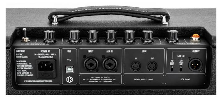
In addition to the input for the guitar, there is also an AUX input, as well as MIDI interfaces (in/out) and a mono output, for example, to send the signal to the FOH or to a recorder. The output can be switched between pre- and post-amp, and a ground lift can also be activated.
