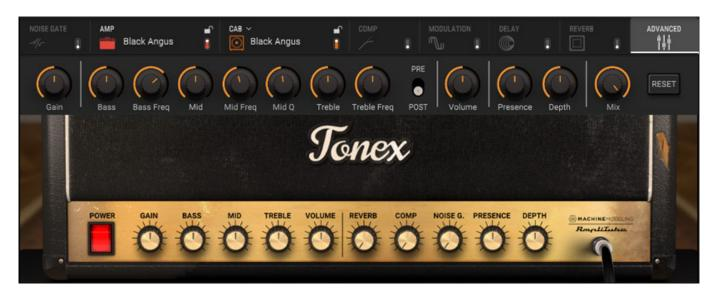
The upper area shows the signal path with the amp and cab, as well as the effects. The virtual button ADVANCED allows you to access the parameters for the amp, such as gain and filter (see figure above).
