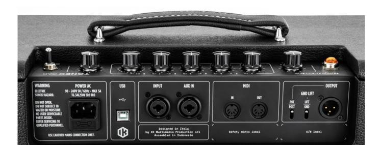
In addition to the input for the guitar, there is also an AUX input, as well as MIDI interfaces (in/out) and a mono output, for example, to send the signal to the FOH or to a recorder. The output can be switched between pre- and post-amp, and a ground lift can also be activated.
