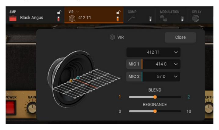
The cabinet can be selected automatically to match the amp, or you can choose a different one (see figure above), allowing you to specify the exact speaker type, microphones, and microphone placement in a dialog box.
