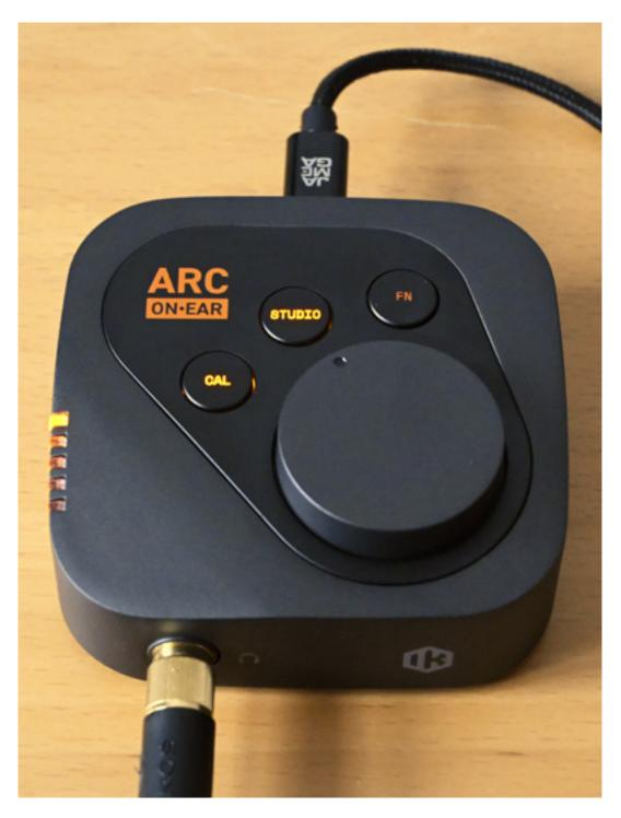
On the top of the ARC ON·EAR, there is a large control for the headphone output level, buttons for activating headphone calibration and studio simulation, and a function button whose function can be defined via the software. The output level is controlled in the analog path, so there is no reduction in resolution.
