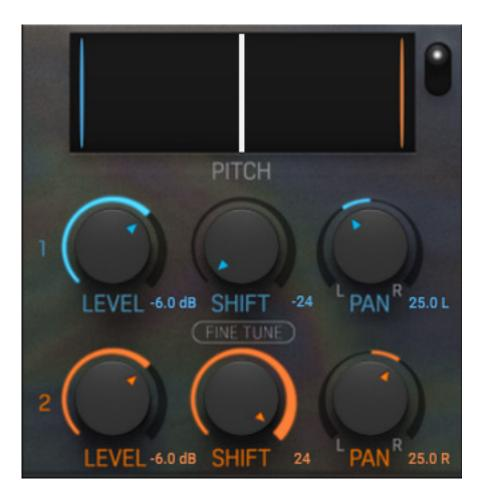
No modern reverb effect would be complete without a shimmer effect. With Prism Reverb, two frequency shifts of up to two octaves are possible. Here, you can adjust the level of the frequency-shifted signal, the frequency shift, and the stereo panorama. A virtual button allows you to fine-tune the frequency. This processing section can also be switched on or off and is graphically visualized.
