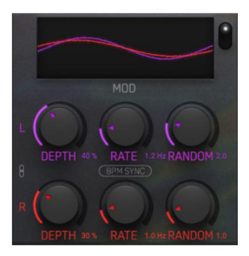
In the MOD section, you can add amplitude modulation to the effect path for each channel. The modulation index, modulation frequency, and a random factor can be independently set for each of the two channels. The rate can also be synchronized to the tempo of the host software.
