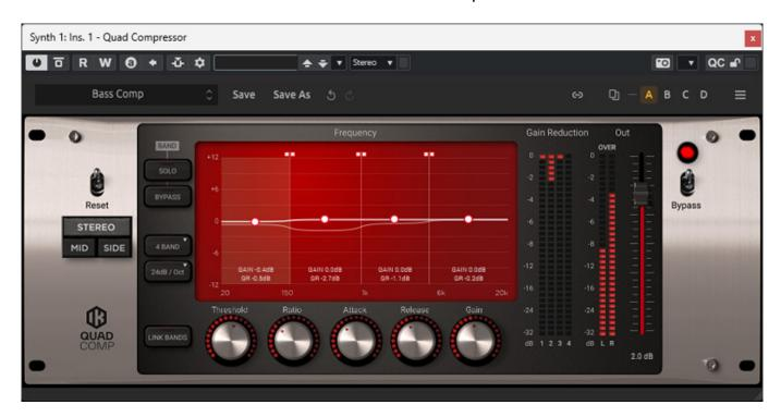
Multiband dynamic plug-ins are also available, such as the four-band processors "Quad Comp" and "Quad Limiter" and, appropriately, there is also a "Quad Image"
