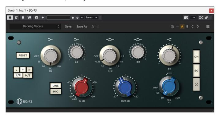
The EQs from Neve are also represented in the bundle as simulations of the 1081 equalizer and 1073 preamp EQ. There is also a simulation of the API 550A with three and four bands with the "EQ PA" and "EQ PB" and a simulation of the API 560 with the "EQ G".
