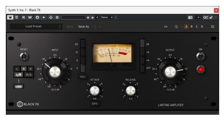
With the "Black 76" there is also a simulation and interpretation of the FET-based limiting amplifier UA 1176 (see illustration above). With the "White 2A", a plug-in
