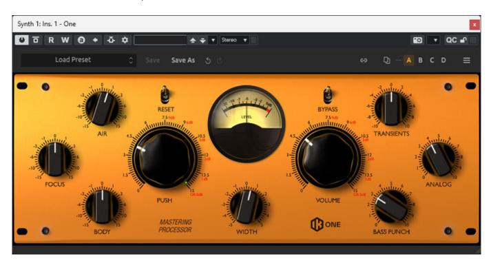
One has been available in T-RackS for some time and is specifically designed for mastering. It combines equalizers (Body, Focus, Air) with a compressor (Push), a stereo base width change (Width) with the option of influencing transients, adding spectrum components as in analogue devices (Harmonics) and a low-end booster. There are also other special mastering plug-ins, such as the Brickwall Limiter, Stealth Limiter, or the Master EQ 432.
