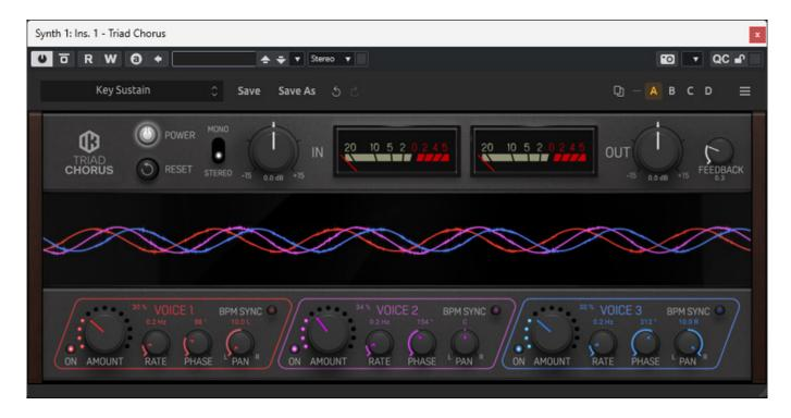
With the update 6.1 of T-Racks, which was released in early November 2024, the Triad Chorus (see figure above) is also available. It offers three chorus voices that can be individually adjusted in intensity, rate, phase and stereo panorama. It is also possible to sync them to the DAW tempo.
