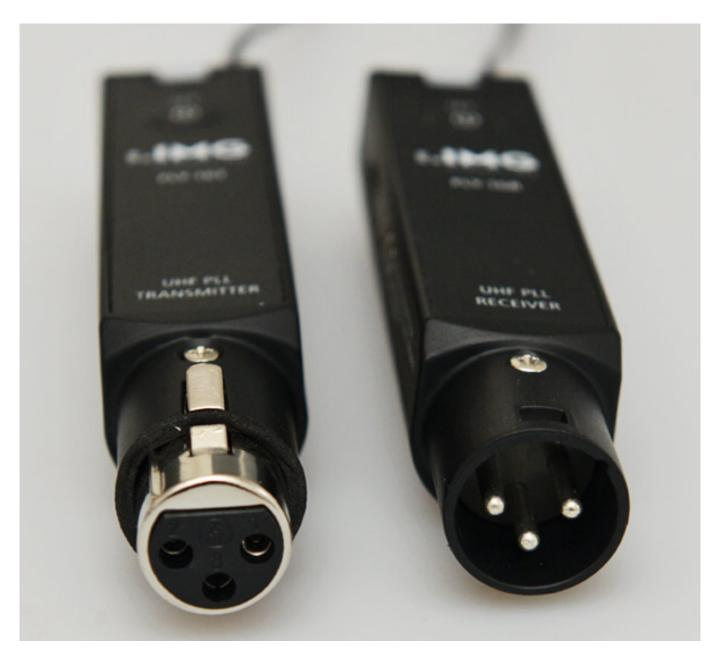
For simultaneous usage of multiple paths, two frequency groups with seven (0, 2, 4, 9, C, E, F) or nine (0, 1, 2, 3, 6, 7, 8, B, C) intermodulation-free channels are recommended. The first instruction manuals specify other frequency groups.
