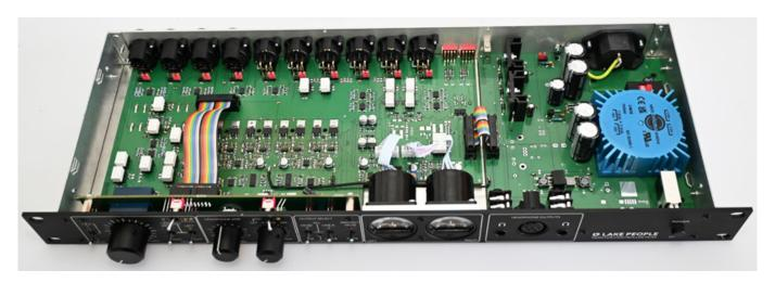
In February 2025, we already had the opportunity to test a pre-production model, which, however, was technically the same as the production model. The housing (483 x 44 x 188 mm) is made of stainless steel, and the front panel is made of three-millimeter aluminum. The integrated power supply (115/230 V, switchable
