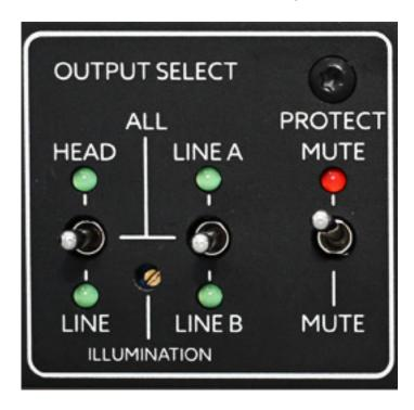
The output section features two three-way switches for line/headphones and line A/B. In the center position, both functions are active. There is also a switch for mute and a status LED in case a protective circuit is activated. Incidentally, there is a delay before the headphones are switched on, and the MC50 also features a temperature monitor to protect the device.
