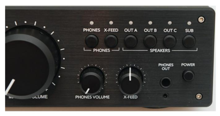
On the right side, you can switch the monitoring playout paths, namely the three monitor paths and the subwoofer playout path. Here, too, the three outputs can be operated in an alternating or multiple mode. This switchover is done by pressing and holding the OUT A and OUT B buttons.
