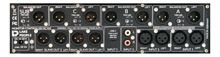
First of all, let's look at the outputs. There are three balanced (XLR jacks) stereo outputs and a switchable subwoofer output (mono, XLR jack). Furthermore, two stereo slave outputs (XLR jacks) are available, which are buffered but not regulated. All outputs offer a maximum level of +26 dBu and an output impedance of  $< 1~\Omega$ . The headphone output on the front panel is available as a 3.5 mm stereo jack, as well as a 6.3 mm stereo jack.
