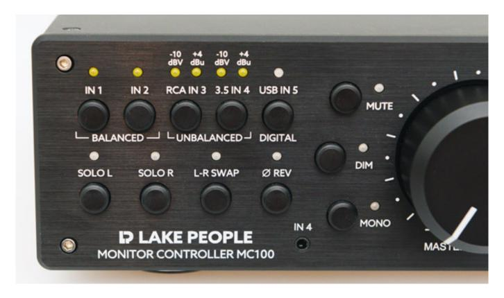
Below that, there are switches for solo left and right, channel swap, and phase swap. On the left side of the volume knob, which is gridded in the standard version (41 grid points), the output signal can be switched to mono, muted (not on the headphones), and dimmed by -20 dB using buttons.
