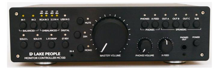
Now for the operation via the front panel controls. At the top left, the input sources can be selected. There are two different selection modes: mutual selection and multiple selection with the summation of the input sources. This can be toggled by pressing and holding the IN 1 and IN 2 buttons. The sensitivity of the unbalanced inputs (RCA on the rear and 3.5-mm jack on the front) can be adjusted between -10 dBV and +4 dBu. This is done by pressing and holding the RCA IN 3 or 3.5 IN 4 buttons.
