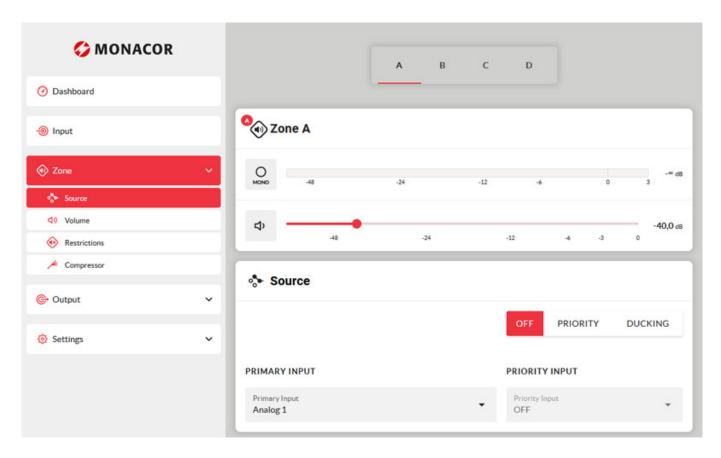
The PA-4125DX supports 4 zones (A ... D). The user can select a zone at the top of the dialogue. Afterwards, the first of 4 settings can be selected in the menu (source, volume, restrictions and compressor).
