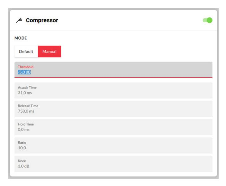
A compressor is also available for each zone. In 'Default' mode, the user can set the threshold. The remaining parameters are set to standard values, i.e. no level adjustments. In addition to the threshold value, the user can also adjust parameters for the compressor in 'Manual' mode, e.g. attack time, release time, hold time, compression ratio and knee point.
