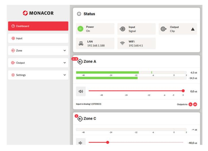
The dashboard (see image above) gives you an overview of the status of the device including virtual faders for the output level and bar graph displays. There is a menu section on the left for selecting various dialogues. In these dialogues, it is possible to select corresponding dialogue sections for the respective zone or for certain features.
