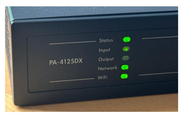
The device is operated completely via the built-in HTML5 web server. There is also an Ethernet connection on the rear panel for integrating it into a local network as well as a 2.4 GHz WLAN which operates as an access point or as a client. The device is delivered in access point mode. Initial configuration is done using a standard password.
