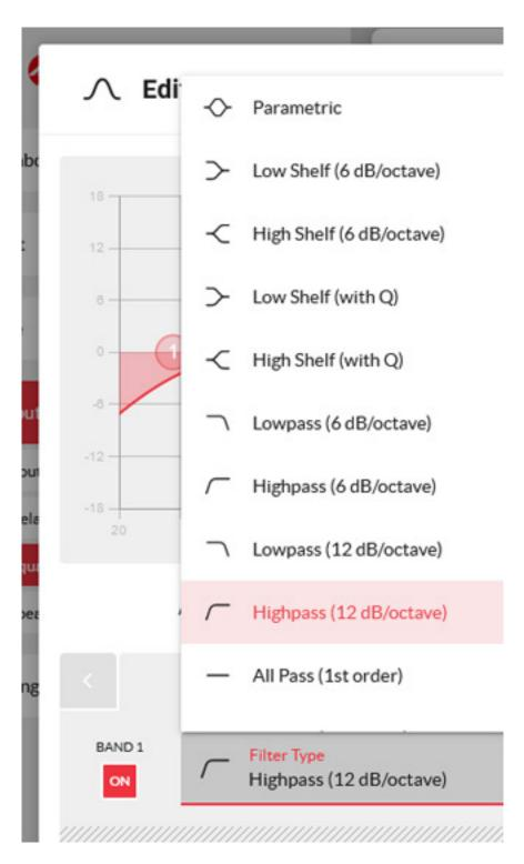
The user can adjust gain, Q and filter frequency, depending on the selected type of filter.
