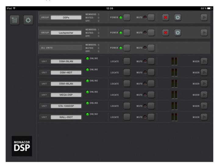
The iPad app provides the same features as the DSP controller software from MONACOR. It is also possible to create device groups. However, the display is designed to match the typical iPad functionality and thus varies slightly from the display of the DSP controller software.
