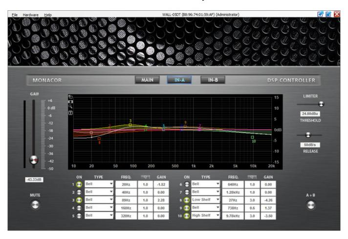
The view Input offers additional options. The values can be imported for both channels via the A+B button. The internal DSP provides a peak limiter with adjustable threshold and an adjustable reset speed (10 to 100 dB per second).
