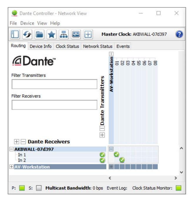
It features an audio resolution of 16 to 32 bits with sampling rates from 44.1 to 96 kHz. The WALL-05DT features two inputs for the Dante network. These input signals can be mixed via the internal DSP. The Dante controller displays these two inputs for every speaker which can be routed to any output in the network (see image above), even to two different Dante audio players or to one stereo source.
