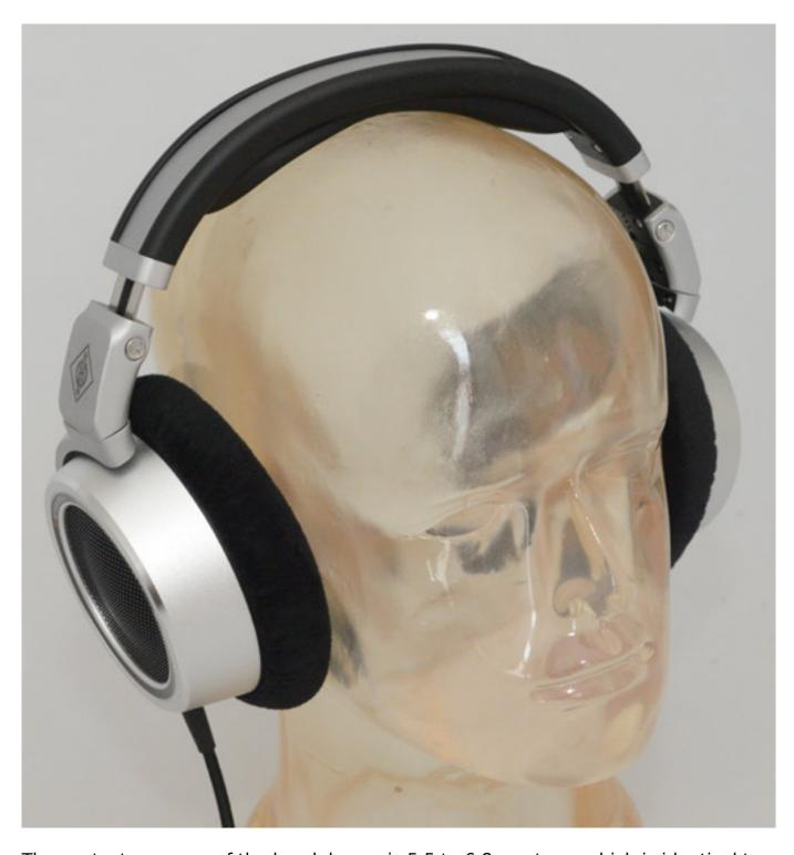
The contact pressure of the headphones is 5.5 to 6.8 newtons, which is identical to the NDH 20. In general, the headphones do not differ in terms of wearing comfort. They are extremely comfortable to wear, even during very long mixing sessions. The ear pads generously enclose the ears. The NDH 30 weighs 352 grams, making it slightly lighter than the NDH 20 (390 grams).
