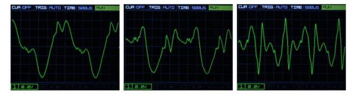
Let us first take a look atthe FOLD knob, which is used to adjust the strength of the wavefolder (see figure above from the knob position slightly above medium to maximum). The behavior is typical of wavefolders in a synthesizer.
