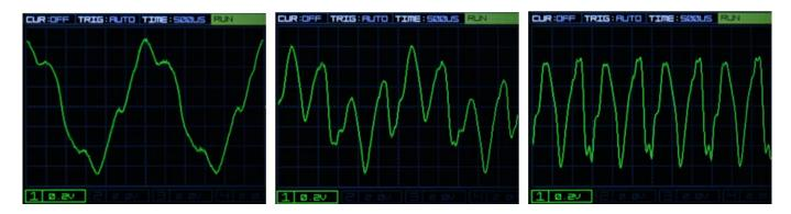
The PURA parameter performs full-wave rectification (see figure above), so that depending on the controller position, the negative portion of the waveform is added in reverse. At the maximum setting, you can observe that the frequency is doubled.
