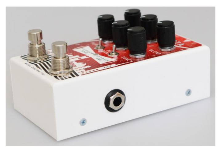
On the right side of the pedal, there is another 6.3-mm jack socket for connecting an expression pedal with a TRS plug. The input impedance is 1 Megaohm and the output impedance is about 100 ohm. The input no clipping range is 500mVpp to 9Vpp, based on selected GAIN position.
