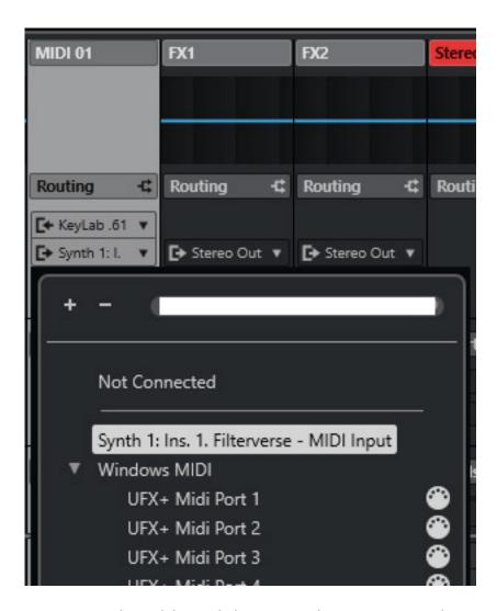
For example, with Steinberg's Cubase or Nuendo, you can create a MIDI track and then assign the inputs and outputs (see figure above). In this example, an Arturia KeyLab 61 controls the filter verse, which has been integrated into a track with a virtual synthesizer.
