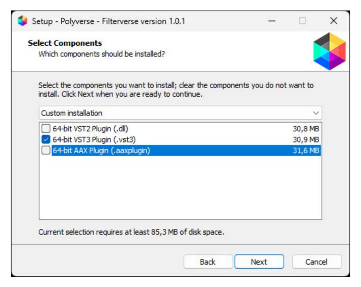
Installation is done using an installer with options for the various plug-in formats.
