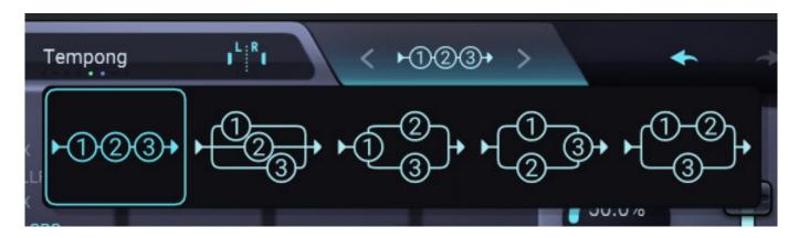
Three filters can be used simultaneously, which can be connected in different ways (see figure above): in series, in parallel, or in mixed variants.
