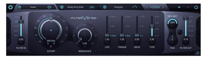
The GUI and the parameters offered adapt to the selected filter type. The knob not only allows you to adjust the output level but also to set a dry/wet ratio between the processed and original signals, as well as the stereo panorama. Mid/side processing is also possible using the "M/S" button.
