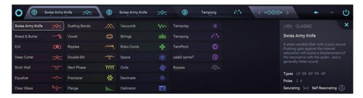
The three filters can be selected using the tabs at the top. You will then see a filter selection on the left and a short description of the filter with some key data on the right (see figure above).
