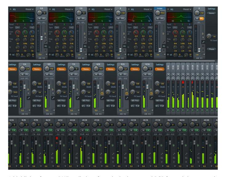
A highlight of many RME audio interfaces is the integrated DSP for real-time control of incoming audio signals in the form of flexible routings for recording, mixing, and monitoring. In addition, effects such as the EQ, dynamics, reverb, and delay are available for each channel. The TotalMix software exclusively tailored for this purpose can be downloaded free of charge for both Windows and Apple operating systems from the manufacturer's download page.
