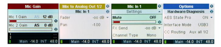
But even without this hardware, all the necessary functions can be set on the device using the detailed display and precise rotary controls. For example, frequently used parameters such as gain, input, and system setup, are clearly displayed in different colors without the need for cumbersome submenu selection.
