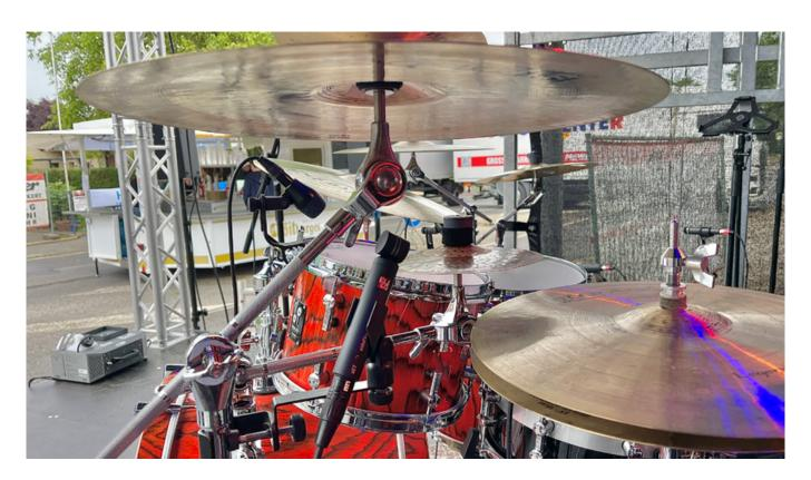
The sE7 sideFire variant also offers interesting options for drum sets. The side capsule arrangement allows the microphones to be optimally positioned - even in confined spaces. When mixing a support act on a local stage, the unusual capsule orientation allows for interesting positioning options.
