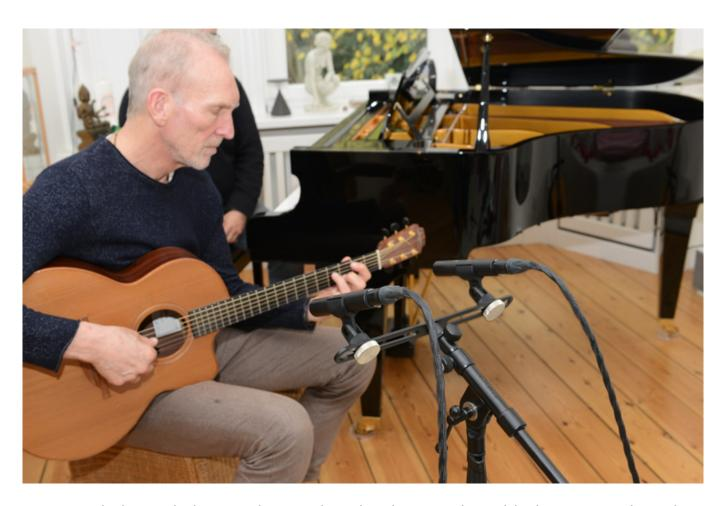
We recorded grand piano and acoustic guitar in a session with the sE8 omnis and other contenders. What is immediately obvious is the excellent bass response. It allows for a good balance between bass, mids and highs. Another point that stuck out was the excellent transient response, especially when miking acoustic guitar. To test that further we recorded some percussive sounds (like jangling silverware). Yes, the sE8 omnis are also very suitable for percussion.
