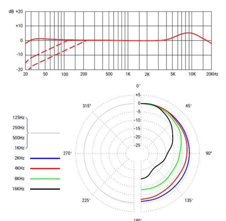
sE specifies the frequency range between 20Hz and 20kHz and the frequency plot (at 180 degree incidence) exhibits the usual bump (about 5dB) around 9kHz.
