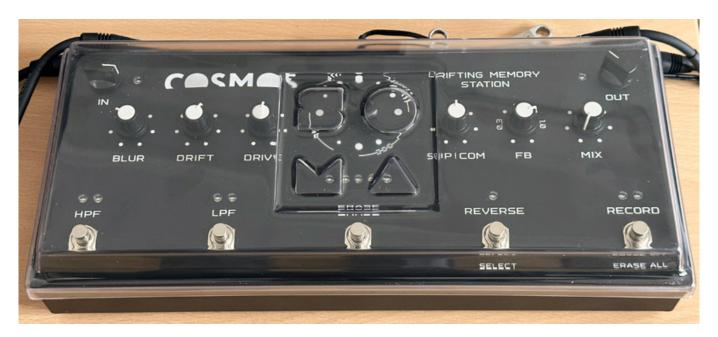
SOMA also offers a matching cover for the COSMOS, which still allows access to the connection jacks. The device can remain connected when the cover is placed. A transport bag and cotton textile cover are also available as accessories.
