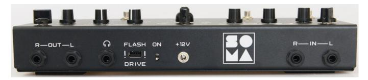
A USB 2.0 socket can be used to connect a FAT32-formatted USB stick to load the firmware. This does not necessarily require an update, but rather there are different firmware versions for different application scenarios. If a firmware file is located in the root directory of the inserted USB stick, will be loaded by pressing the RECORD button and the turning on the device.
