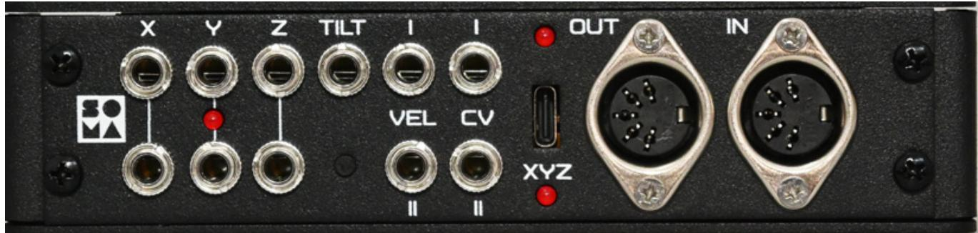
The connection between Flux and the breakout box is made using a USB-A/USB-C cable. The LED between the XYZ jacks indicates the power supply, and a status LED above the USB jack indicates a successful USB connection. In addition to the USB jack, there is a five-pin MIDI-In and a MIDI-Out jack.
