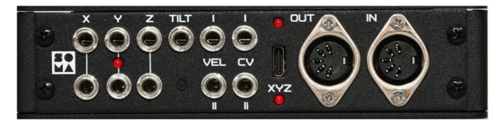
The connection between Flux and the breakout box is made using a USB-A/USB-C cable. The LED between the XYZ jacks indicates the power supply, and a status LED above the USB jack indicates a successful USB connection. In addition to the USB jack, there is a five-pin MIDI-In and a MIDI-Out jack.
