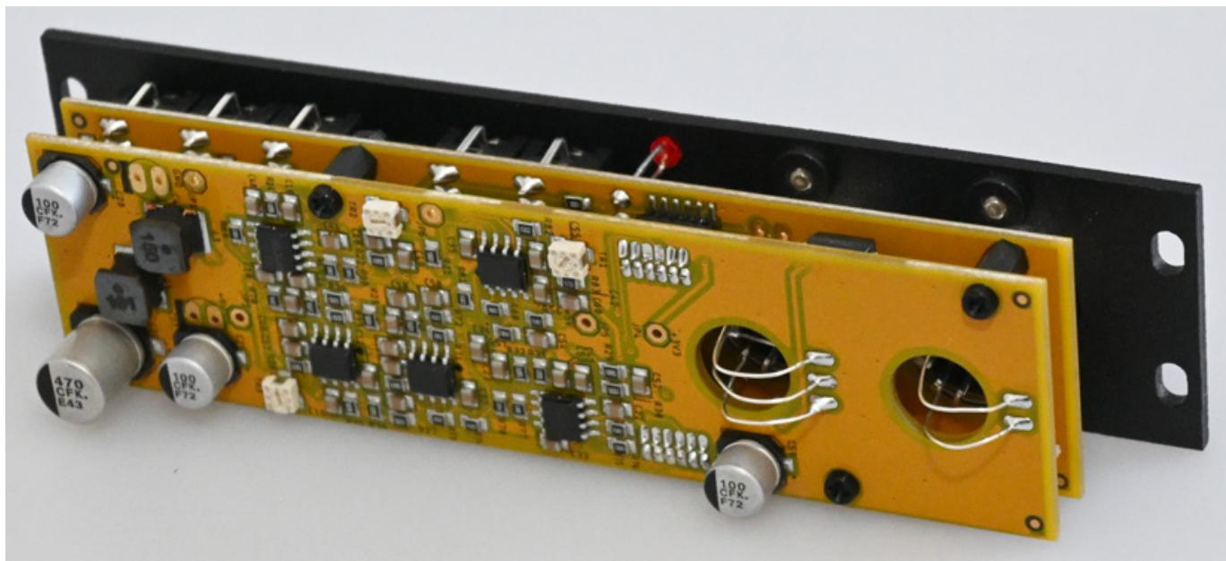
The Flux Breakout Box is a Eurorack module with a width of 6U, which is supplied in a mini metal case. It is connected directly to the Flux via a USB cable and is also supplied with voltage for Operation from there. When installed in a Eurorack, it does therefore not need to be connected to the power supply there. The Flux firmware version 1.6 or higher is required for operation.
